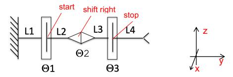
(a) Complete the DH table for this given manipulator (ignore L1, L4). Remember that joints  $\Theta$ i should be along the z-axis, and links Li along the x or z-axis.
