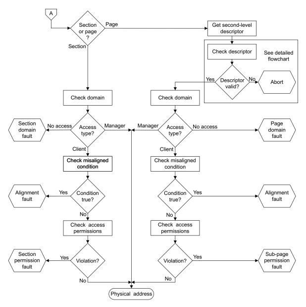
Figure 6-3 Translation table managed TLB fault checking sequence, part 2
