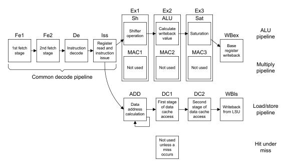
Figure 1-7 Pipeline progression of an LDM or STM operation
