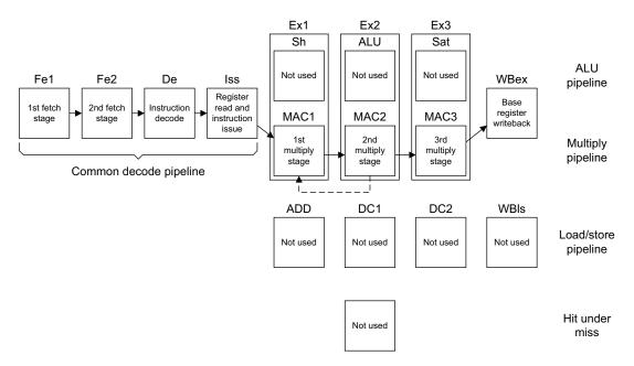
Figure 1-5 Pipeline for a typical multiply operation
