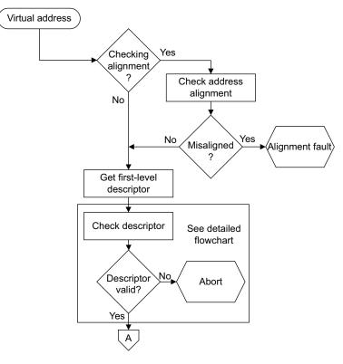
Figure 6-1 Translation table managed TLB fault checking sequence, part 1
