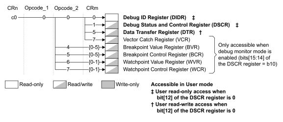
Figure 13-2 shows the arrangement of the Debug registers in CP14:
