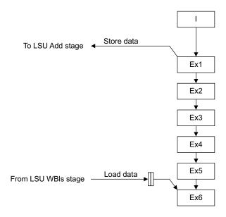
Figure 11-8 Coprocessor data transfer
