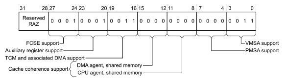
Figure 3-17 Memory Model Feature Register 0 format
