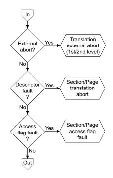
Figure 6-2 Descriptor checking for Translation table managed TLB fault checking, level 1 and level 2
