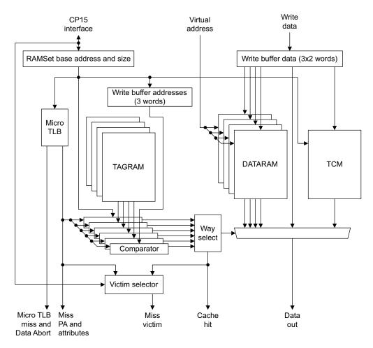
Figure 7-1 Level one cache block diagram
