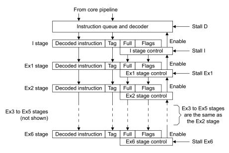
Figure 11-3 Coprocessor pipeline
