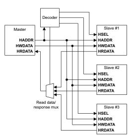
Figure 8-7 AHB-Lite block diagram
