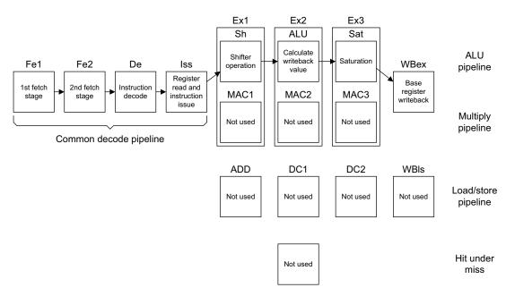
Figure 1-4 shows a typical ALU data processing instruction. The processor does not use the load/store pipeline or the HUM buffer are not used.
