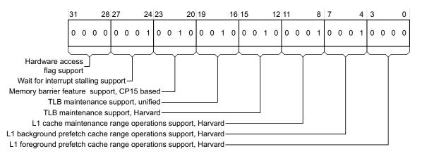
Figure 3-19 Memory Model Feature Register 2 format
