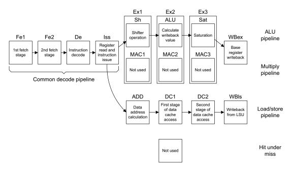
Figure 1-6 shows an LDR or STR operation that hits in the Data Cache.
