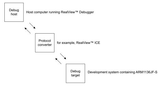
Figure 13-1 Typical debug system
