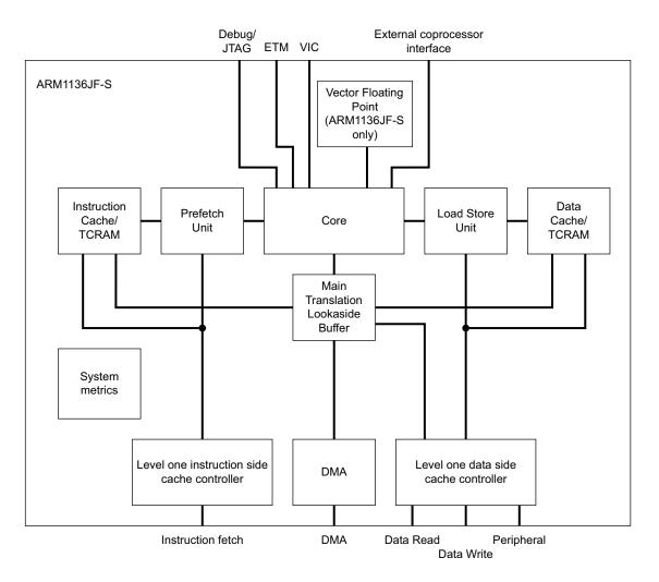
Figure 1-1 ARM1136JF-S processor block diagram
