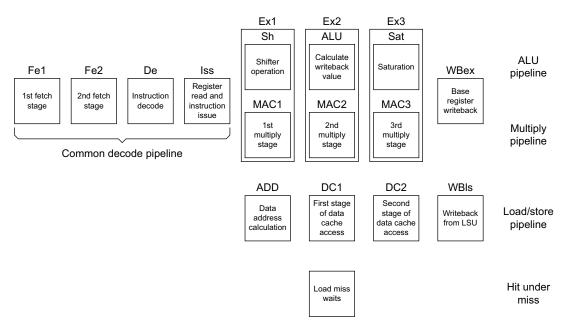
Figure 1-3 Typical operations in pipeline stages
