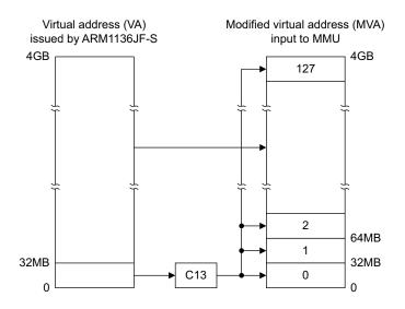
Figure 3-58 Address mapping using CP15 c13
