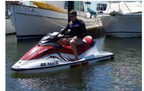
REVski Electric conversion of Sea-Doo Jet Ski: 4-TEC, 96V, 50kW, 7.6kWh, 30min. drive-time.
