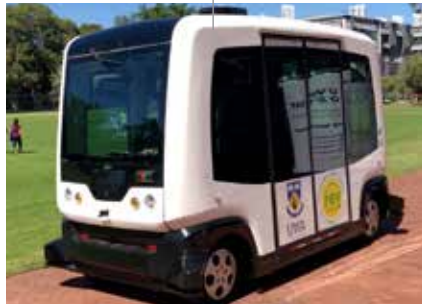
The nUWay fleet—four Autonomous Electric Shuttle Buses 48V, 15.36kWh, 8 Lidars, 2 cameras, IMU, RTK-GNSS.
