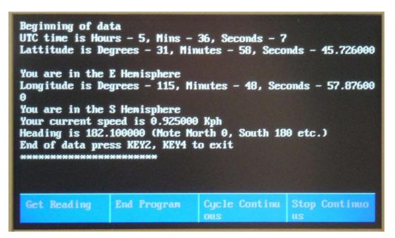
Figure 7 - One reading of the getGPSdata test-demo program
