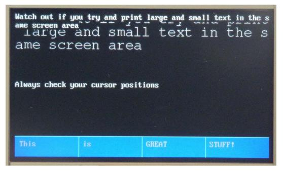
Figure 9 - The clash between large and small text on screen is visible. The same message was printed to sceen for both text sizes both cursor positions started at (0,0)
