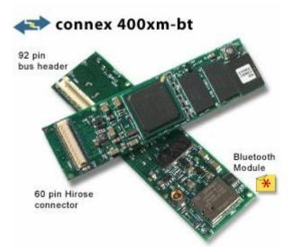
Figure 5 - The Gumstix connex used in the EyeBot M6 (Gumstix connex 400xm-bt 2008)
