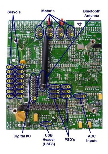
Figure 3 - The Bottom of the EyeBot M6 illustrating the I/O connectors
