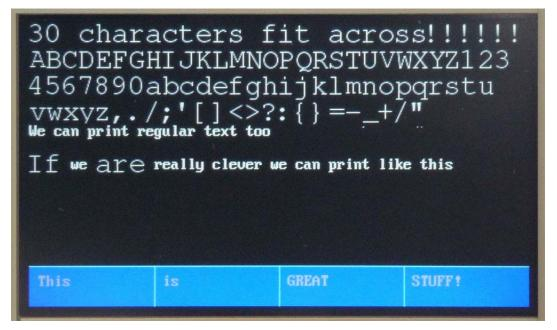
Figure 10 - A screen shot of part of the test-libM6lcd program, both font sizes are displayed simultaneously
