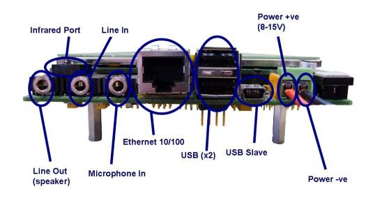
Figure 4 - The side of the EyeBot M6 illustrating power ports and modern connectivity devices
