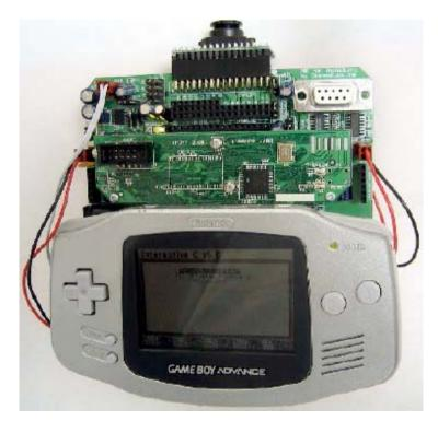
Figure 1 - The XBC Controller (LeGrand et al. 2005)
