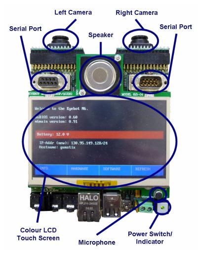
Figure 2 - Top side of EyeBot M6 illustrating hardware
