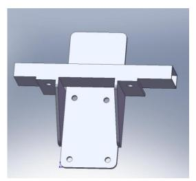
FIGURE 32: AIR-CONDITIOING COMPRESSOR BRACKET
