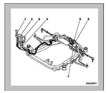
FIGURE 24: EHPAS SYSTEM CONFIGURATION (OPEL MOTORS CO.)
