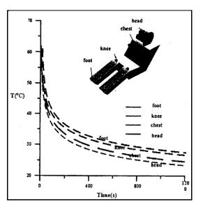
FIGURE 5: THE AIR TRANSIENT TEMPERATURE NEAR THE PASSENGER, (CHIEN ET AL., 2008)
