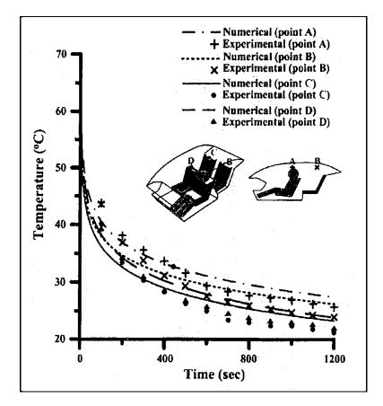
FIGURE 11: TEMPERATURE VS TIME PLOT OF EXPERIMENTAL & NUMERICAL DATA
