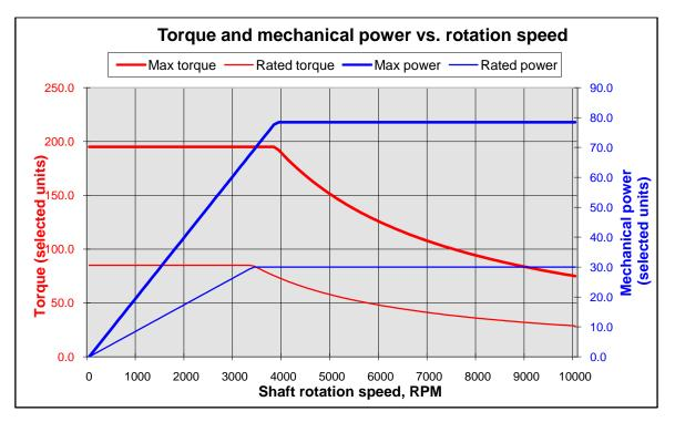
FIGURE 21: AC INDUCTION MOTOR PERFORMANCE CUVE (METRICMIND, 2008)
