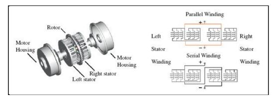
FIGURE 8: ELECTRIC WHEEL MOTOR CONFIGURATION(YANG AND LO, 2008)
