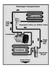
FIGURE 3: TYPICAL AUTOMOTIVE A/C SYSTEM CONFIGURATION, (CHILLYWILLYS.ORG, 2008)
