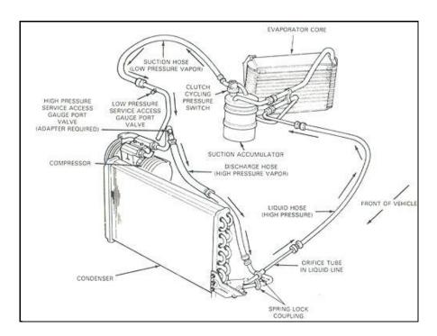
FIGURE 10: COMPLETE AIR-CONDITIONG CIRCUIT DIAGRAM, (EDMUNDS, 2008)
