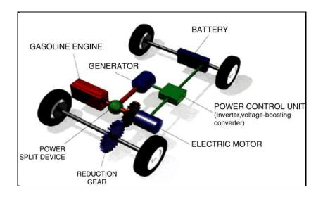
FIGURE 2: TYPICAL HYBRID CONFIGURATION, (PROKHOROV, 2008)
