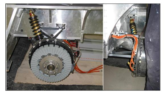
Figure 19: Wheel motor (HybridAuto.PTY.LTD, 2006)
