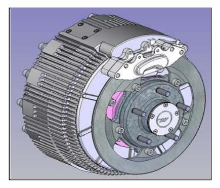
FIGURE 27: WHEEL MOTOR DIRECT DRIVE (WAVECRESTLABS, 2008)
