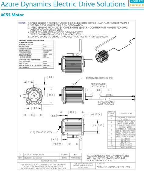
FIGURE 36: AC55 TRACTION MOTOR DIMENSIONS
