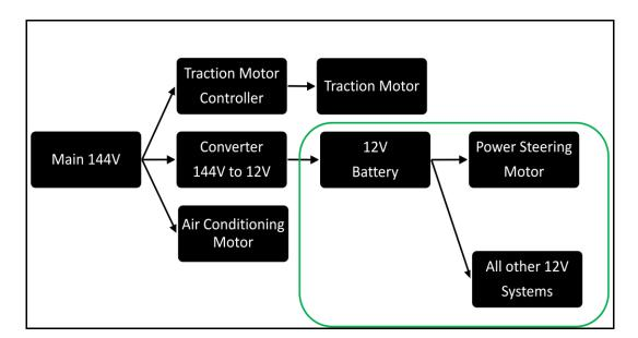
FIGURE 23: EHPAS ENERGY SUPPLY DIAGRAM
