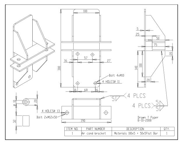
FIGURE 33: COMPRESSOR MOUNTING BRACKET
