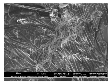
**Figure 20:** Fibrillation and Fibre Pullout Marks
