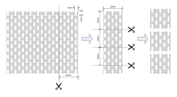
Figure 8: Kevlar Cutting Technique
