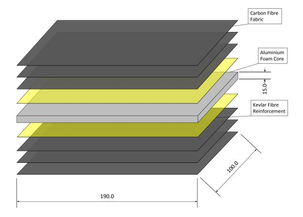
Figure 10: Composite Sandwich Structure Assembly
