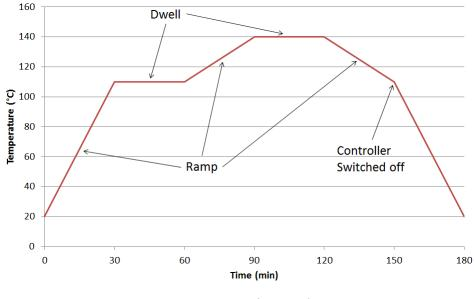
Figure 12: Curing Cycle
