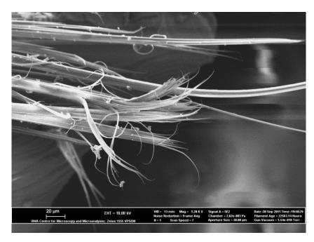
Figure 19: Multiple Split Break of Kevlar Fibres
