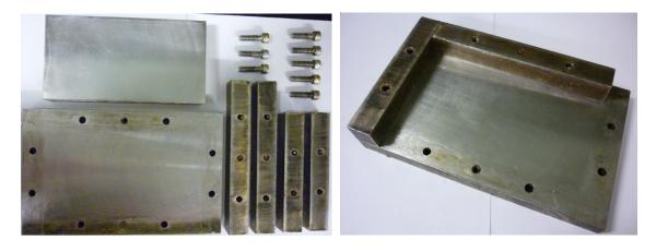
Figure 6: Parts of the Mould Assembly
