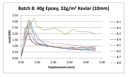
Figure 15: Typical Load vs. Displacement Curves
