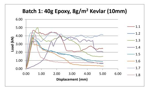
Figure 16: Load vs. Displacement with Multiple Peaks
