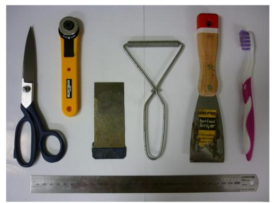
**Figure 22:** Experimental Equipment (From left to right: Robuso scissors, OLFA rotary cutter, flexible applicator, steel roller, scraper, toothbrush, steel rule)
