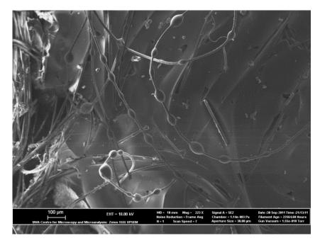
Figure 21: Kevlar Fibres Wet with Epoxy
