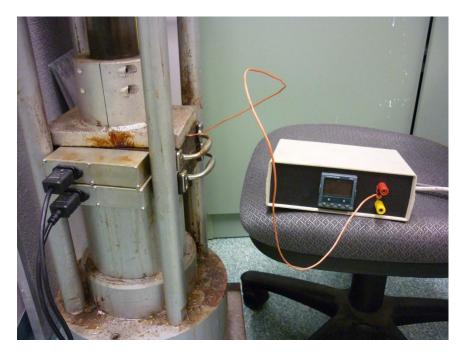
Figure 26: Hot Platen Air Press and Eurotherm 2416 PID Controller
