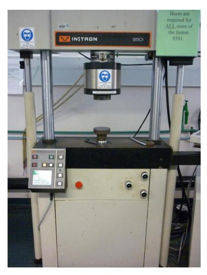
Figure 24: Instron 8501 Testing Machine
