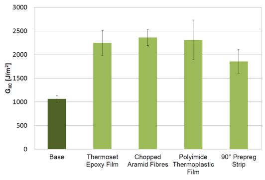
Figure 5: Comparison of reinforcement techniques (Bond et al. 2011)
