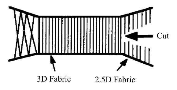
Figure 4: Fabrication of 2.5D fabric (Sohn & Hu 1998)
