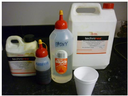
Figure 23: Epoxy Resin, Hardener and Mixing Cup
