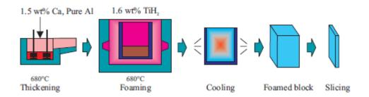
Figure 1: Manufacturing Process of Alporas (Akiyama et al. 2000)
