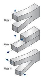
Figure 3: The 3 modes of fracture (NDT Resource Centre, 2011)
