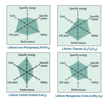
Figure 10 The relative merit of various Li-ion chemistries [13].
