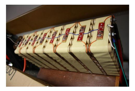
Figure 8 One of the accumulator packs with BMS modules installed.
