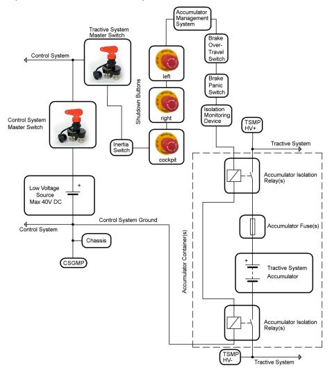
Figure 4 An overview of the shutdown circuit [4].
