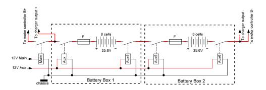
Figure 18 The new design of the tractive system accumulator.
