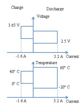
Figure 11 Safe Operating Area of LiFePO<sub>4</sub> battery cell.
