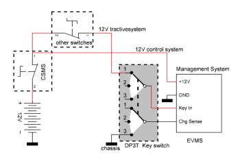
Figure 21 Interface the drive and charge interlock
