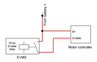
Figure 23 Interface between EVMS and motor controller
