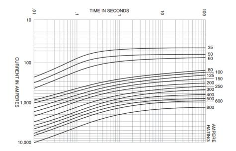
Figure 16 Time-Current Characteristic Curve of ANN fuses [19].
