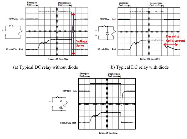
(c) Typical DC relay with diode and Zener Figure 26 Operate & Release Dynamics Coil V&I [22]
