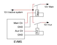
Figure 19 The additional relays on the EVMS terminals
