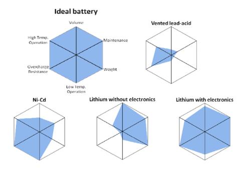
Figure 9 Relative merits of various battery technologies [11].
