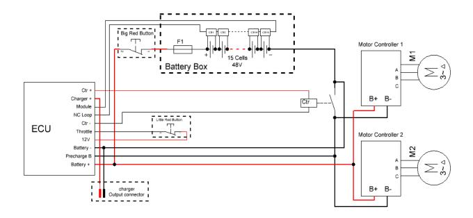
Figure 6 The schematic of the electrical system of the prototype vehicle.
