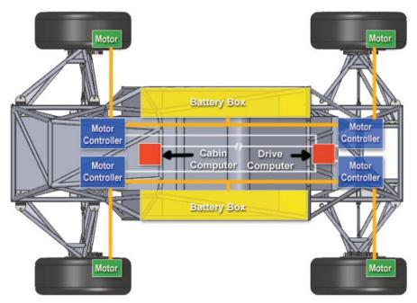
Figure 7 Top views of next generation Formula SAE-Electric showing component locations [7].
