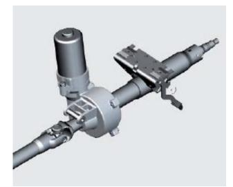
Figure 4: An electric motor (the vertical cylinder) provides steering assistance by driving the steering column [7].
