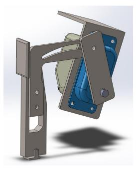
Figure 11: CAD Drawing of an initial brake-by-wire design concept.
