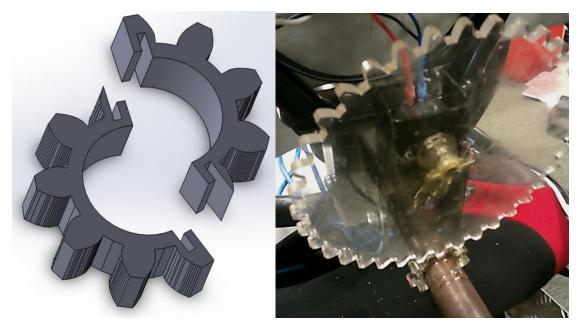
Figure 21: Split gear design.
