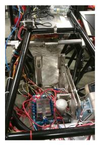
Figure 33: The nose of the vehicle which houses most of the low-level autonomous system. The brake mechanism is shown on the right with numerous electronic circuits housed in the blue box on the left.
