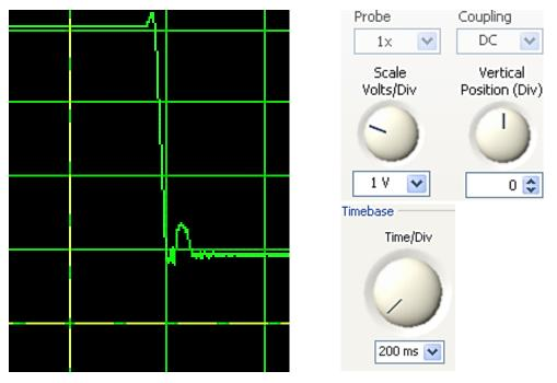
Figure 14: Measurement of the throttle hall sensor from full acceleration to no acceleration.
