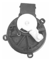
Figure 5: A hall sensor assembly that is attached to a brake pedal mounting to allow computer assisted braking. Two hall sensors are present to allow for redundancy [11].
