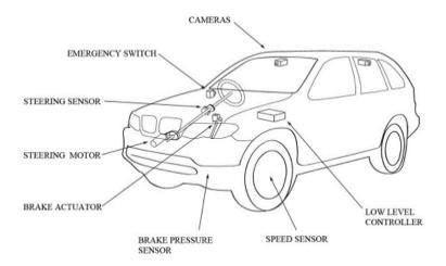
Figure 3: Overview of the BMW X5 modified to drive-by-wire [1].
