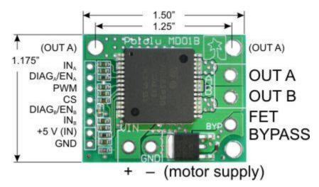
Figure 23: The Pololu VNH2SP30 motor controller breakout board [31].
