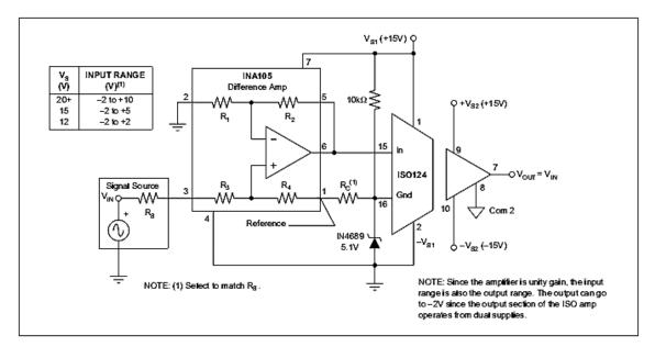
Figure 15: The standard setup for the ISO124 under a single positive rail voltage available on the input side [26].
