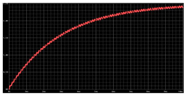
Figure 18: Output signal of the circuit in Figure 17 with a 50% input PWM duty cycle.
