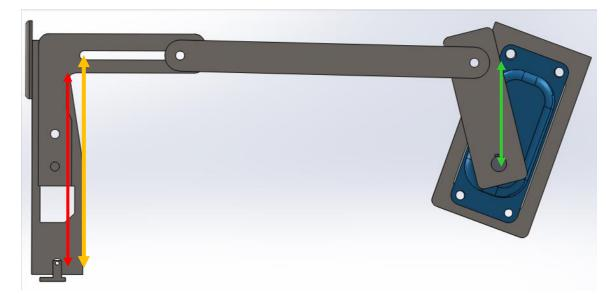
Figure 13: Measurements for design of the brake-by-wire linkage.
