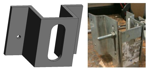
Figure 20: The initial bracket design to house the steering feedback sensor (left), with the final bracket shown on the right.
