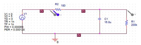
Figure 17: OrCAD PSpice simulation environment for the throttle-by-wire digital to analogue filter.
