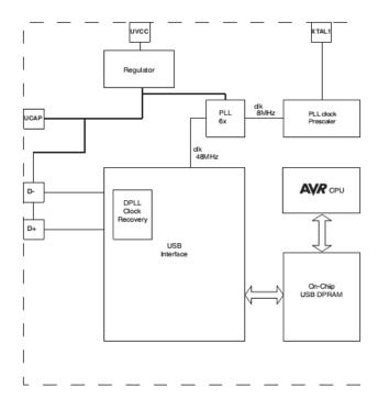
Figure 32: The diagram of the USB communication circuit located inside the ATMEL16U2 on the Arduino board ([40], page 185).
