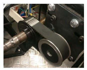
Figure 28: The constructed actuator for the autonomous steering system.
