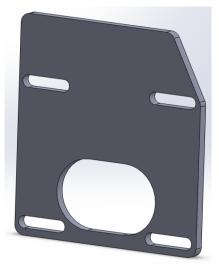
Figure 25: A drawing of the slotted bracket used to mount the steering actuator.
