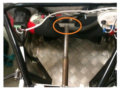
Figure 19: The chosen area to mount a sensor for steering position feedback.
