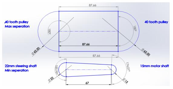
Figure 26: A Solidworks sketch used to determine the maximum and minimum belt lengths possible for use in the steering system.
