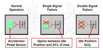
Figure 6: Operational states of engine throttle of Toyota's 2<sup>nd</sup> generation Electronic Throttle Control System-intelligence [14].
