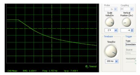
Figure 34: Voltage decay caused by the capacitance of the SSPS-105 servomotor.
