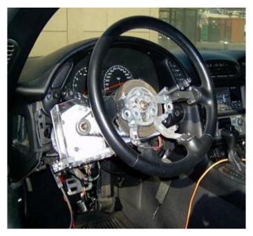
Figure 8: Modified steering setup for actuation by an electric motor [16].
