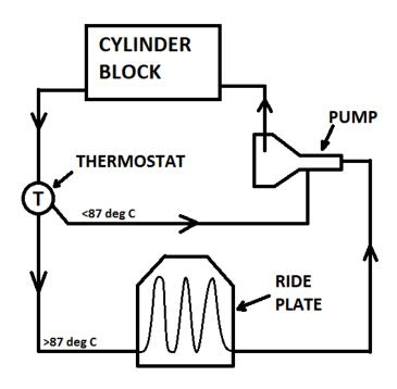
Figure 1: Existing cooling system for the internal combustion engine on the Sea-Doo jetski
