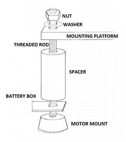
Figure 13: Schematic of the forward supporting point of the auxiliary mounting platform for the REVjet
