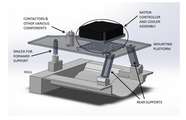
Figure 18: Model image of the auxiliary mounting system designed for the REVjet
