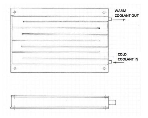
Figure 7: Sheetmetal cooling plate
