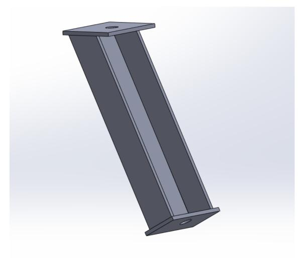
Figure 12: Support for auxiliary mounting platform for mounting components within the REVjet
