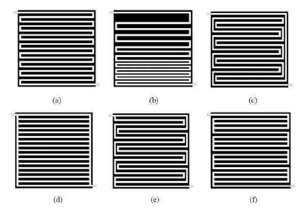
Figure 5: Cooling flow configurations investigated by Choi et al. (2008)
