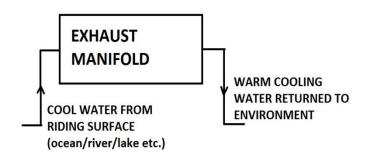
Figure 2: Representation of open loop system cooling configuration as used in the exhaust system of the Sea-Doo jetski
