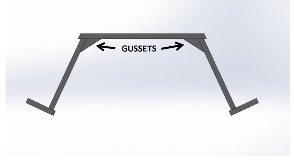
Figure 10: Flat bar bridge with gussets to increase stiffness
