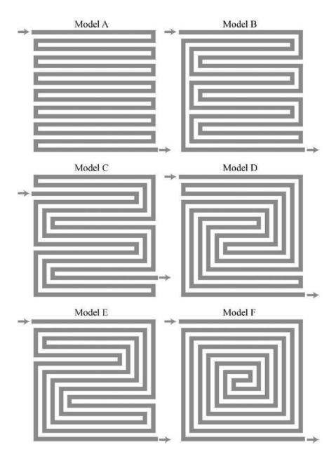
**Figure 6:** Configurations of flow channels in cooling plates analysed by Yu et al. (2009)
