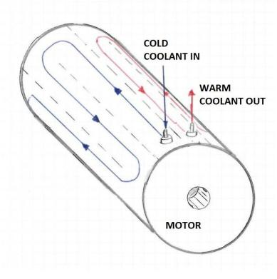
Figure 3: Illustration of the electric motor and its cooling jacket for the REVjet
