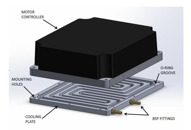
Figure 14: Motor controller and cooling plate assembly designed for the REVjet
