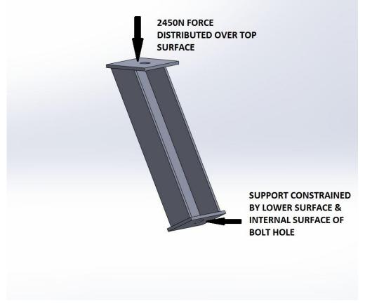
Figure 15: Force and constraint conditions applied during stress analysis of the auxiliary mounting platform supports
