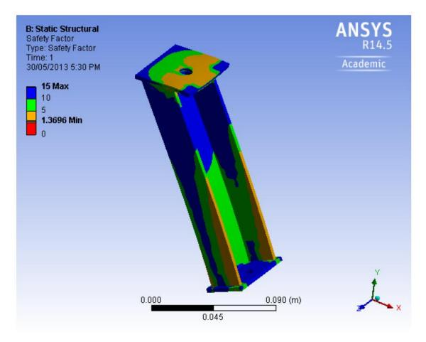
Figure 16: Safety factor analysis for the auxiliary mounting platform supports.
