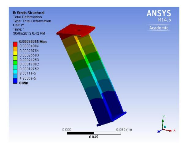
Figure 17: Results of deformation analysis performed on supporting members for the auxiliary mounting platform
