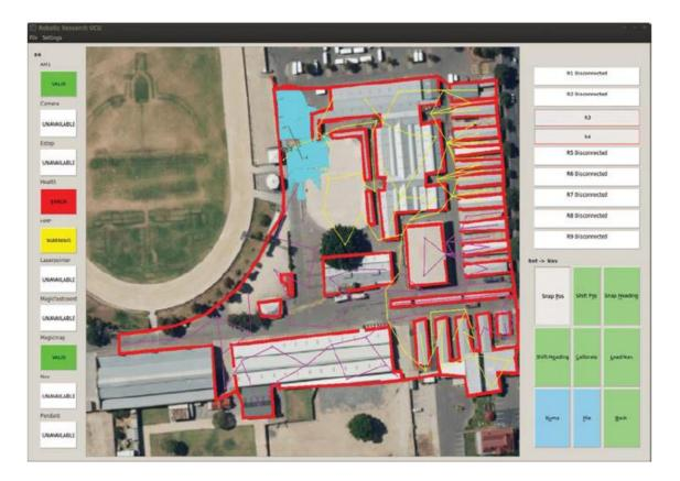
**Figure 1.4** A screenshot from the system developed by the RASR team for MAGIC2010. Shown on the right hand side is the robot status feedback mechanism. The central display shows the robots exploring the environment with overlayed robot position (Lacaze, et al., 2012).
