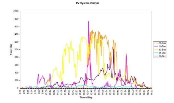
Figure 2 - Power Output Profile for a PV System over 1 day
