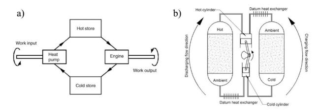
Figure 12 - a) simplified flow diagram of a PHES system, b) simplified schematic of an energy storage system
