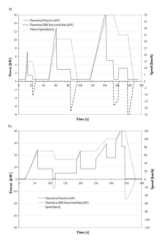
Figure 3-7: The city a) and highway b) drive cycle model output with speed profile, estimated energy demand and RBS energy recovery profile
