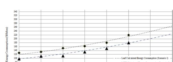
Figure 7-2 Measured and extrapolated energy consumption over a speed range of 60 to 130 km/h.
