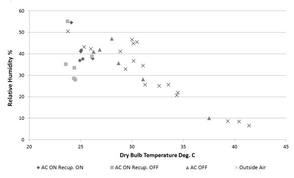
Figure 4-12 Outside air and passenger compartment mean temperatures and humidity over the six test days under different driving configurations
