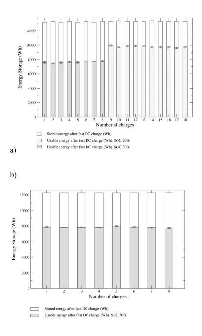
Figure 6-2 Stored and usable energy during a series of fast-DC charges. a) Nissan Leaf stored and usable energy. b) MiEV stored and usable energy over the charge cycles.
