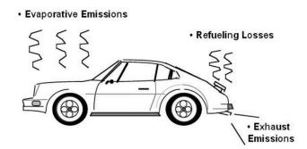
Figure 1-2 Emission sources on combustion engine motor vehicle [9]
