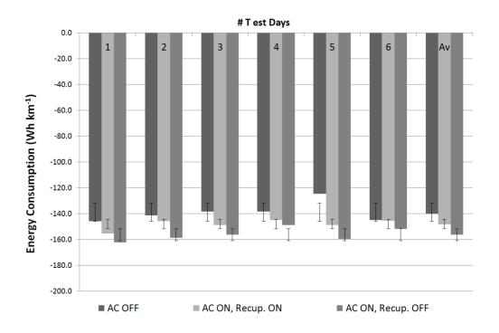
Figure 4-8 The Ford Focus EV average energy consumption over the six testing days and the overall average (in Wh km<sup>-1</sup>) with standard deviation error bars
