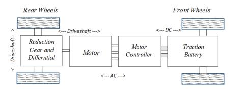
Figure 3-3: Schematic diagram of the drive train of the MiEV
