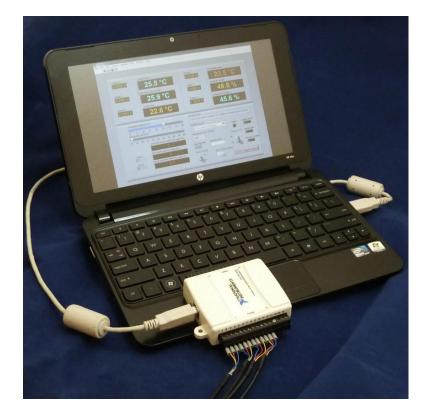
Figure 4-7 The custom designed logging system
