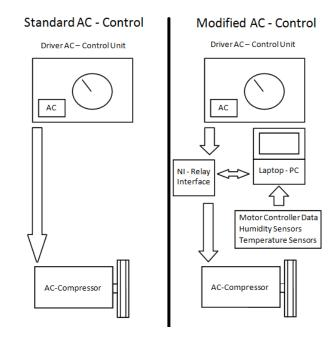
Figure 4-5 Schematic of a standard AC control system (left), and the modified AC control system (right) developed for the experiment
