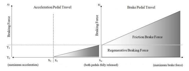
Figure 3-4: Diagram to illustrate RBS brake force in respect to acceleration pedal travel (A) and brake force in respect to brake pedal travel (B) assuming a vehicle speed larger than 16 kmh<sup>-1</sup>
