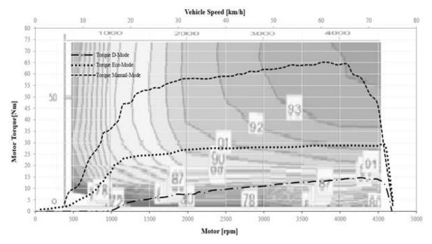
Figure 5-8: Measured data from deceleration tests overlayed onto a section of the Nissan Leafs motor and controller efficiency map during the three deceleration scenarios (Background reproduced with permission from Oak Ridge National Laboratory [32] )
