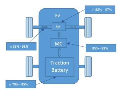
Figure 2-2: EV power train components with typical efficiencies
