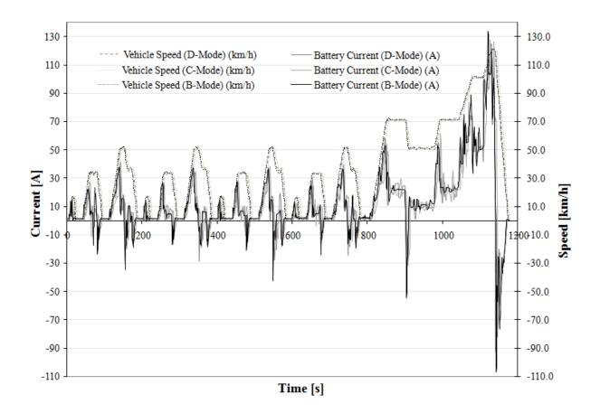
Figure 3-8: i-MiEV speed and current profile during three NEDC drive cycles for modes C, B, and D.
