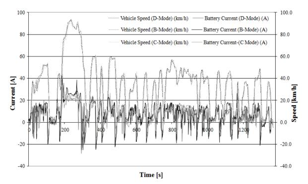
Figure 3-10: i-MiEV speed and current profile during three FTP 75 drive cycles for modes C, B, and D.
