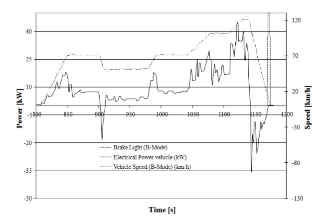
Figure 3-9: The NEDC Highway section speed profile, traction, regeneration power and the short period of the friction brake (brake light) in use below 16 km h<sup>-1</sup> near the end of the highway section.
