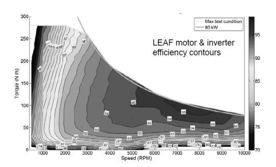
Figure 5-2: A Nissan Leaf efficiency map and overlayed test results at 80kW up to 10,000 rpm Reproduced with permission from Oak Ridge National Laboratory [32]
