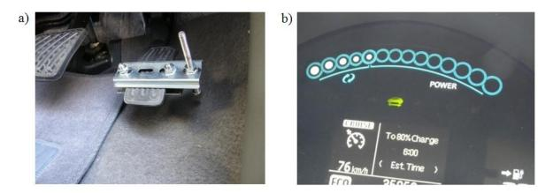
Figure 5-3: (a) An adjustable mechanical pedal stop provided a uniform acceleration demand signal and (b)the vehicle's internal power meter under full recuperation provided driver feedback for the highest deceleration scenario
