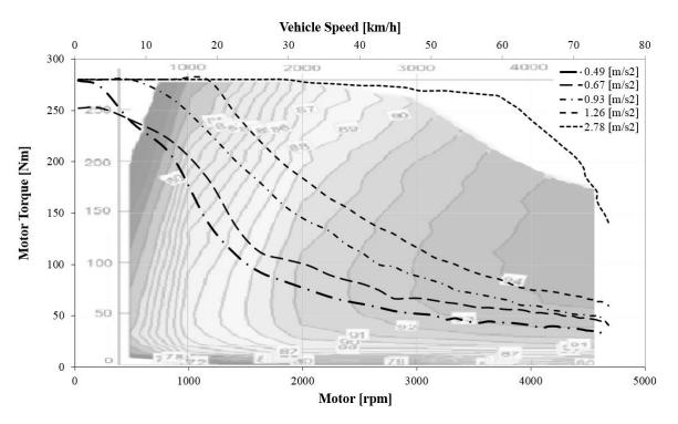
Figure 5-6: Measured data from test drives with five different acceleration rates overlaid onto a section of the Nissan Leafs motor and controller efficiency map (Background reproduced with permission from Oak Ridge National Laboratory [32]
