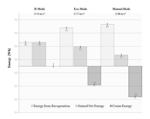
Figure 5-7: Energy recovered during deceleration, cruise and total (net energy) during the series of three decelerations from 70km/h to 0km/h.
