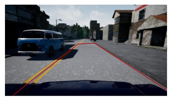
Figure 23: ROI area for vehicle and pedestrian detection
