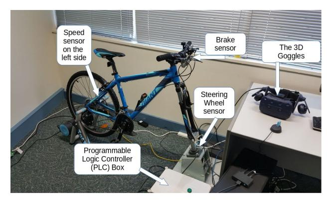
Figure 3.2, The bicycle simulator with the sensors, PLC box and 3D Goggles, (Machiel van der Stelt, 2020).
