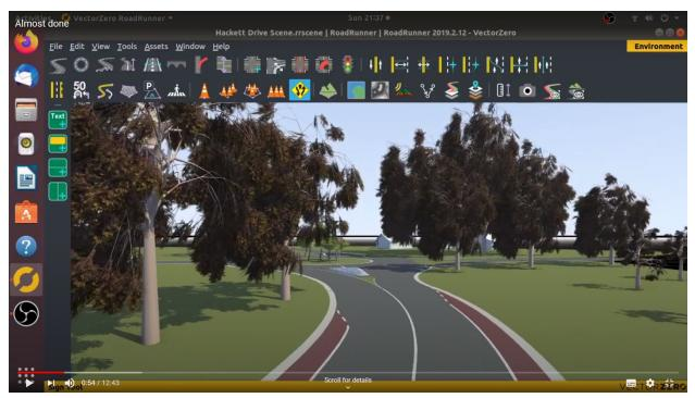
Figure 3.11, the Bicycle lane gradually narrows until it disappears from the road, (Machiel van der Stelt, 2020).
