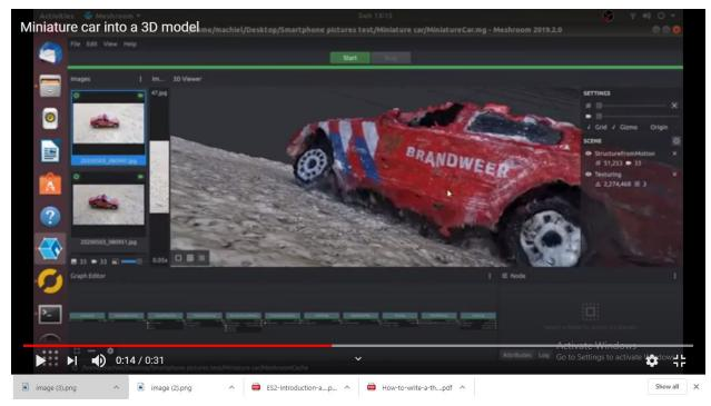
Figure 3.17, Miniature 3D car model produced after pictures were taken and processed in Meshroom, with obvious rendering errors, (Machiel van der Stelt, 2020).
