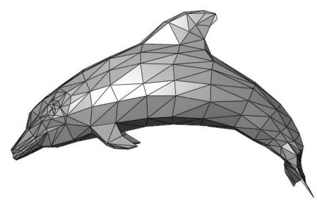
Figure 3.12.1 Polygon 3D Mesh model of a Dolphin, (Wikipedia, 2020).
