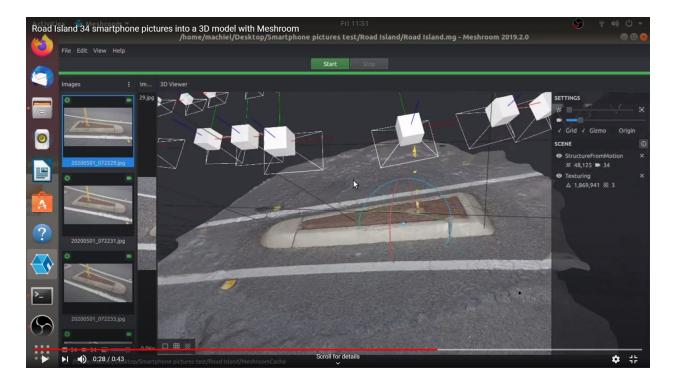
Figure 3.13, A very detailed Road Island after about 20 minutes of rendering in Meshroom with 30+ smartphone pictures, (Machiel van der Stelt, 2020).
