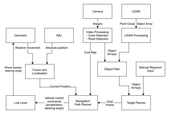
Fig. 8.6 FSAE vehicle ROS node structure.
