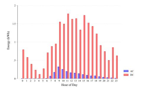
Fig. 10.11 The differences in instantaneous energy delivered by an AC station versus a DC station at each hour of day (CS vs DC).
