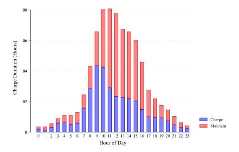
Fig. 10.6 The average vehicle charging times starting at each given hour of day for an AC station.
