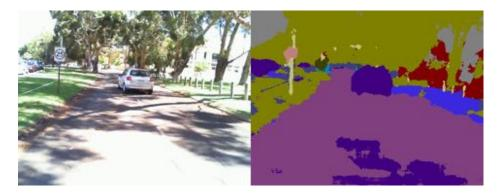
Fig. 5.13 Segmentation results on a road with pronounced shadows.
