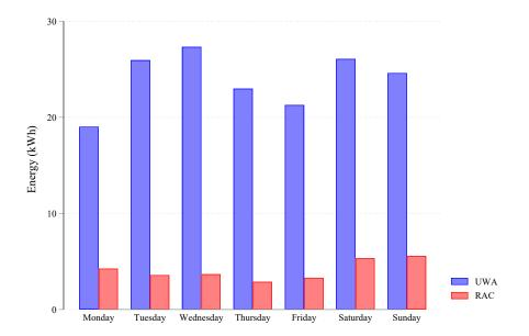
Fig. 10.18 The energy delivered per station per day of week between the UWA (12/11/2014 to 13/10/2017) and the Electric Highway (RAC) (02/03/2016 to 20/09/2016) DC stations.
