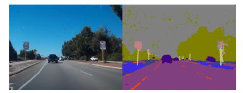
Fig. 2.4 SegNet's input (left) and output (right) for a typical Western Australian road scene.
