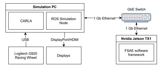
Fig. 8.4 Autonomous driving simulator hardware diagram.
