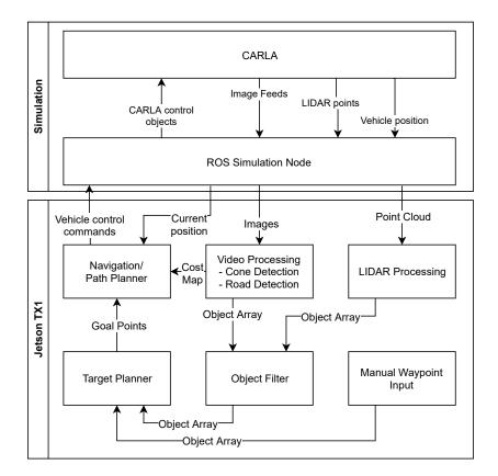
Fig. 8.7 Software framework architecture with CARLA simulator interface.
