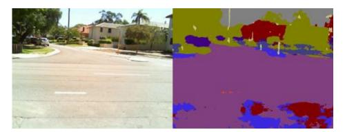
Fig. 5.12 Segmentation results at a road junction.
