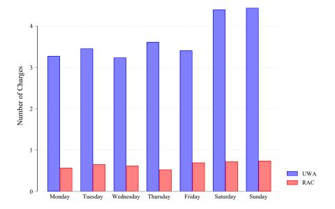
Fig. 10.15 Number of DC charge events per station per day of week between the UWA (12/11/2014 to 13/10/2017) and the Electric Highway (RAC) (02/03/2016 to 20/09/2016).
