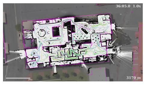
Fig. 4.8 Completed global grid-map with ground truth overlaid in magenta.
