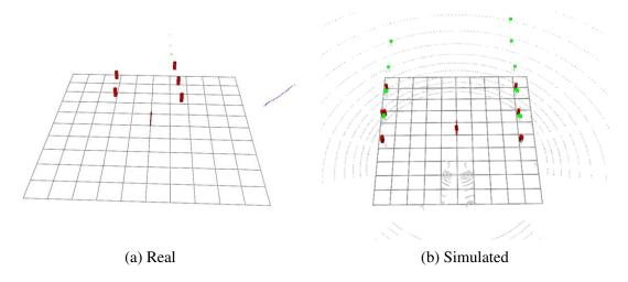
Fig. 7.14 LiDAR cone processing outputs from (a) real and (b) simulated scenarios.
