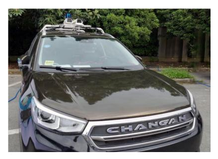
Fig. 1.2 An autonomous car with its sensors visibly mounted on its roof.
