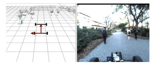
Fig. 7.4 Point cloud generated from the LMS111 (coloured) and the LUX (4-layers, white) (left) and the scene where it was captured (right).
