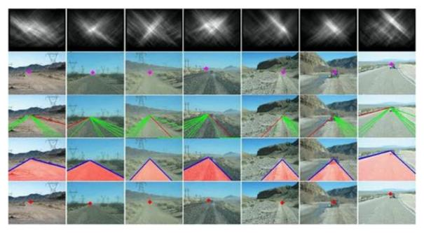
Fig. 2.2 Vanishing point estimation of seven desert road images showing the LASV algorithm. Reprinted with permission from [62].
