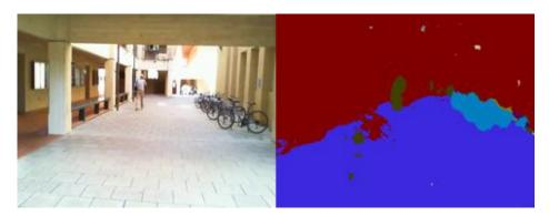
Fig. 5.11 Segmentation results on pavement between faculty buildings.
