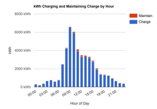
Fig. 9.27 Energy drawn (in kWh) by hour of day stacked with power drawn for charging versus power drawn for maintaining charge.
