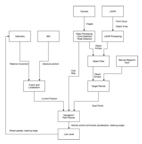
Fig. 7.2 SAE vehicle software framework.
