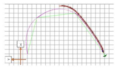
Fig. 7.5 Calculated waypoints on RViz with inputs from (7.2) and (7.3).
