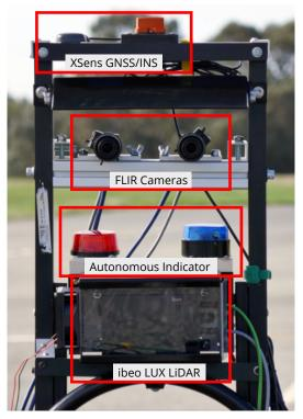
Fig. 8.9 Autonomous FSAE sensor rack.
