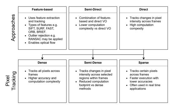
Fig. 3.2 Processing techniques used in VO according to their approaches and their pixel tracking methods for direct approaches.
