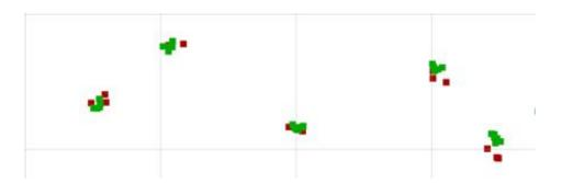
Fig. 8.12 Comparison of LiDAR point clouds from real (green) and simulated (red) scenarios.
