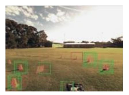
Fig. 7.11 Visual cone detection showing the detected cones in bounding boxes.
