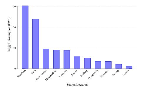
Fig. 10.17 The amount of energy in kWh delivered per day for each DC station from the UWA (12/11/2014 to 13/10/2017) and the RAC (02/03/2016 to 20/09/2016).
