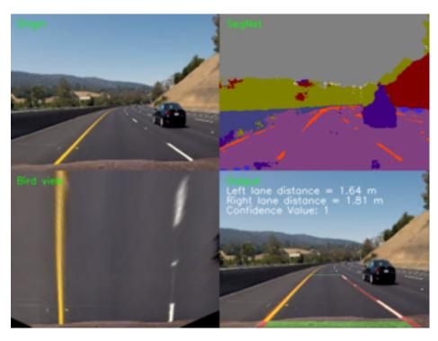
Fig. 5.2 Lane distance measurements with SegNet's output on Udacity's Self-Driving Car Nanodegree recording [139] as the input in "Origin".
