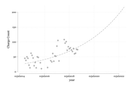
Fig. 9.30 A regression model forecasting the per-month charge frequency on the DC charging station
