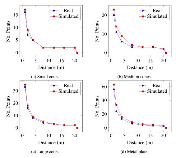
Fig. 8.13 Number of LiDAR points returned by small cones (a), medium cones (b), large cones (c) and a metal plate (d) at varying distances.
