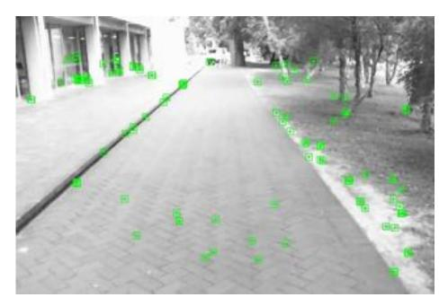
Fig. 4.10 ORB features tracked by ORB-SLAM2 as shown in bounding boxes.
