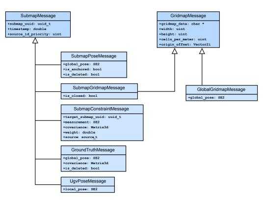
Fig. 4.3 A class diagram showing the MR-SLAM system's message types and their variables.
