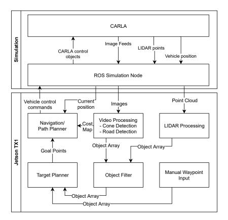
Fig. 7.8 Simulation software framework.
