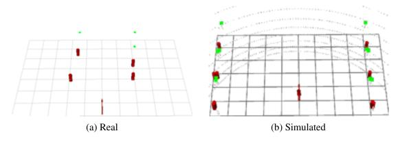
Fig. 8.11 LiDAR-based cone detection results from real (a) and simulated (b) scenarios. The raw LiDAR data is displayed in green, and detected cones are displayed in red.
