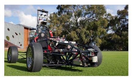
Fig. 1.4 The REV Project's autonomous Formula SAE Electric test vehicle.
