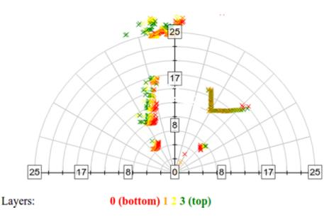
Fig. 5.9 LiDAR plot showing the detected parked vehicles at the position where Fig. 5.8 was captured. The graph axes measure distances in metres.
