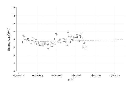
Fig. 9.33 A regression model forecasting the per-month charging energy consumption per charge on the AC charging network.
