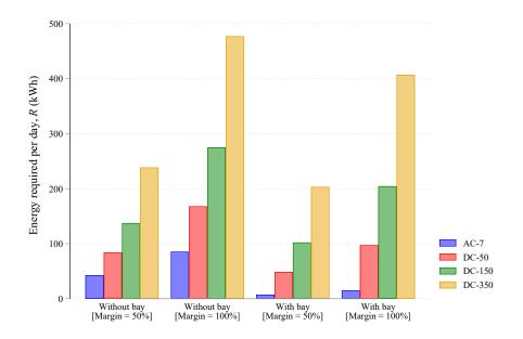
Fig. 10.22 Break-even points for the AC and DC stations' energy delivery in kWh required under scenarios representing with or without bay rentals  $C_B$  (Bay/No bay), with sales margins set at 50% (M = 0.5) and 100% (M = 1).
