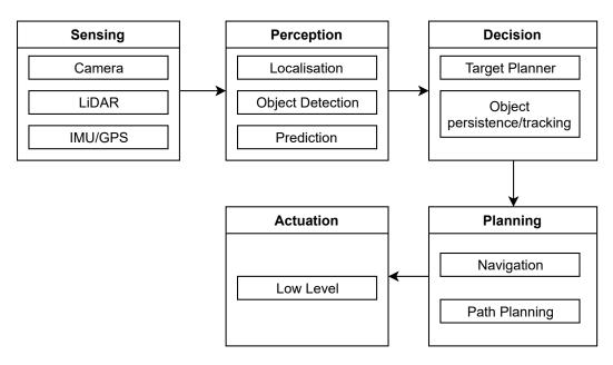
Fig. 8.2 High-level architecture of the Autoware project, adapted from [327].
