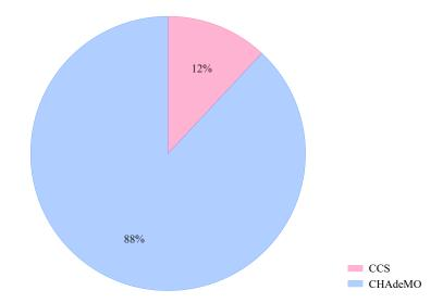
Fig. 10.21 Percentage of connector types used at the UWA DC station (12/11/2014 to 13/10/2017).
