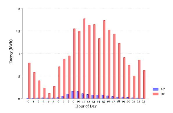
Fig. 9.34 Per-hour energy usage comparison between AC and DC charging stations.
