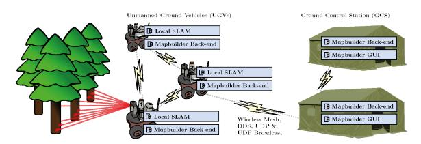
Fig. 4.2 The MR-SLAM architecture and software development diagram showing the software components run on the GCS and UGVs.
