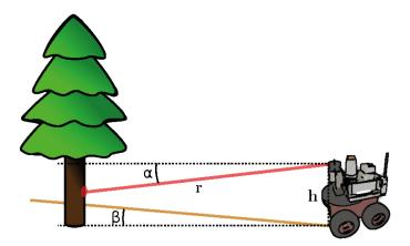
Fig. 4.4 Lengths and angles used for calculating the local SLAM prefilter.
