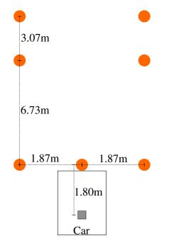
Fig. 5.4 The topological distance between bollards (dots) and the camera on the car (shaded square).
