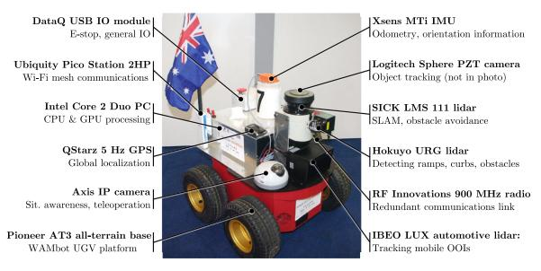
Fig. 4.1 Photo illustrating an single MRS UGV with its hardware modules as labelled.
