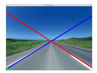
Fig. 2.3 Lane detection with Hough transform performed using OpenCV
