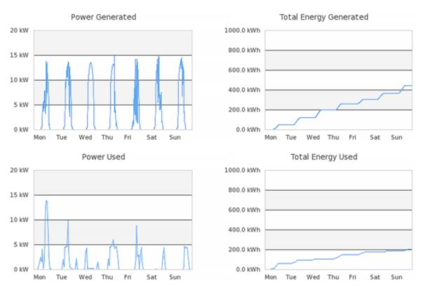
Fig. 9.21 Graphs generated from solar PV data over a typical week.
