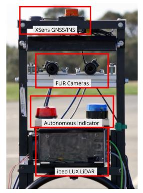
Fig. 7.3 The SAE vehicle's rack-mounted sensors.
