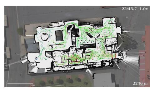
Fig. 4.7 SLAM output showing loop closure between both teams, with the first team about to exit via the southwestern corner.
