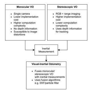
Fig. 3.1 Types of VO approaches as classified by their imagery methods. Visual-inertial odometry is VO that is fused with inertial measurements.
