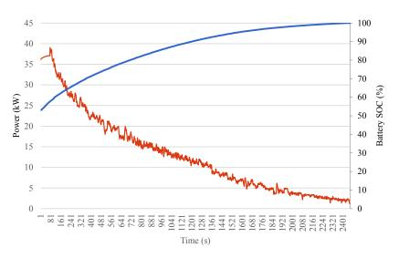
Fig. 10.2 Battery charge rate (kW) in red and State of Charge (%) in blue over time.
