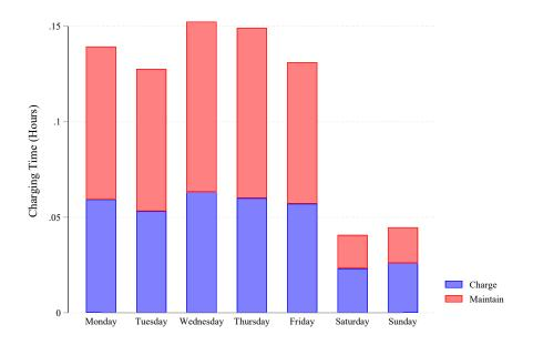
Fig. 10.8 The average vehicle charging times for each day of week for an AC station.
