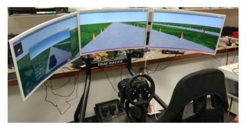
Fig. 8.5 Autonomous driving simulator setup.
