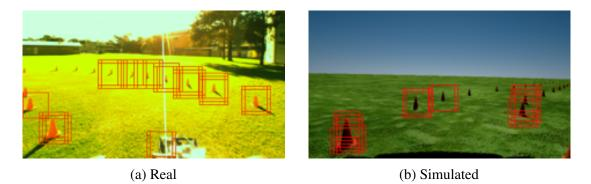
Fig. 8.14 Computer vision based cone detection results from real (a) and simulated (b) scenarios.
