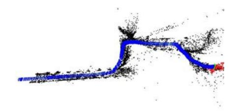
Fig. 4.11 Trajectory measured using ORB-SLAM2 for dead reckoning (blue), previously tracked ORB features (black) and presently tracked ORB features (red).
