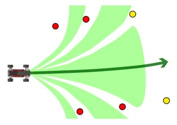
Fig. 7.12 Visualisation of the path planner on cone driving. Immediate cones are red and subsequent cones are yellow; green regions are viable paths.
