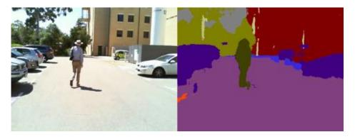
Fig. 4.13 SegNet output from a parking area showing segmented road regions (purple), road markings (orange), and poles (yellow).
