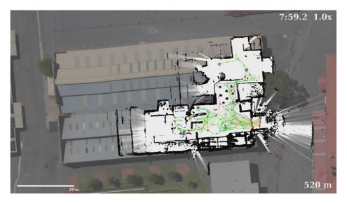
Fig. 4.6 SLAM output showing the UGVs starting at the southeastern corner of the environment.
