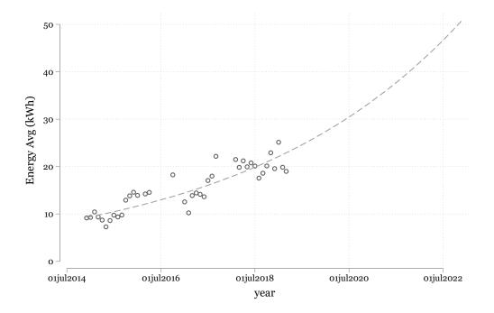
Fig. 9.31 A regression model forecasting the per-month charging energy consumption per charge on the DC charging station.
