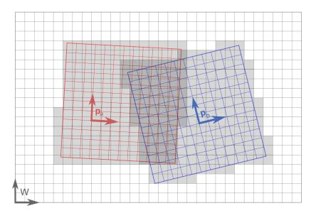
Fig. 4.5 Occupancy grid-map fusion illustrating two submap grid-maps with their origins  $p_a^W$  and  $p_b^W$  to be fused onto the global output grid-map W shown as grey grids.
