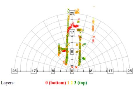
Fig. 5.6 LiDAR plot showing the detected road edges and the bollards' positions from the car where Fig. 5.5 was captured. The graph axes measure distances in metres.
