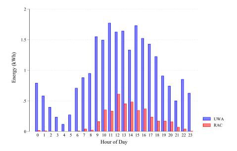
Fig. 10.19 The energy delivered per station per hour of day between the UWA (12/11/2014 to 13/10/2017) and the RAC (02/03/2016 to 20/09/2016) DC stations.
