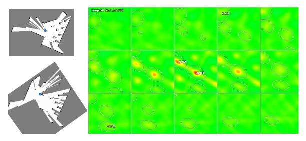
Fig. 4.9 Example of multimodal constraint output with perceptual aliasing. The correlation results for a test area with perceptual aliasing that was caused by repetitive geometry. It shows an overlapping submap pair (left) along with 15 slices through their constraint likelihood volume.
