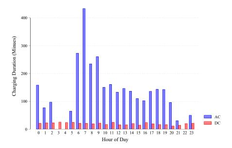
Fig. 10.12 The difference in charging time on an AC station versus a DC station at each hour of day.
