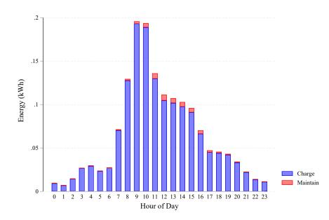
Fig. 10.5 The average energy delivered at each hour of day for an AC station.
