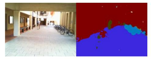
Fig. 4.12 SegNet output showing segmented pedestrian (olive), bicycles (light blue), pathway (blue) and building (red).
