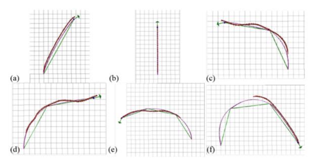
Fig. 7.9 Generated path projections  $M_i$  (red), its ground truth  $D_i$  (purple) and the linear displacements of waypoints (green). [Grid size:  $1 \text{ m} \times 1 \text{ m}$ ]
