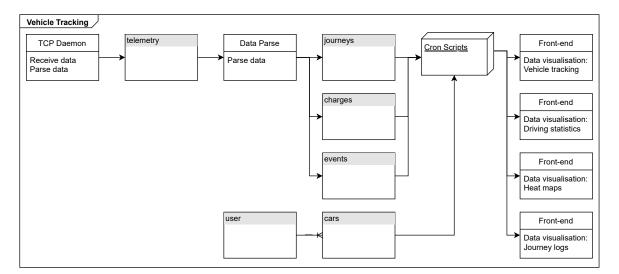
Fig. 9.12 Simplified class diagram showing REView's vehicle tracking system.
