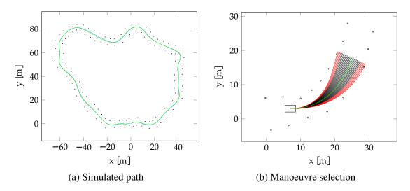
Fig. 6.2 Simulated near-optimal path (a) and manoeuvre selection (b). Black dots represent road delimiters.
