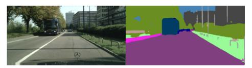
Fig. 2.5 KittiSeg's input (left) and output (right) on the Cityscapes dataset using a Tensor-flow [126] implementation. Reprinted with permission from [127]
