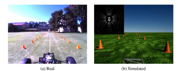
Fig. 7.13 Scenarios used for comparing (a) real and (b) simulated LiDAR and visual cone processing outputs.
