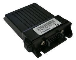
Fig. 9.13 An Astra Telematics AT240 vehicle tracking device used in our vehicle fleet network.
