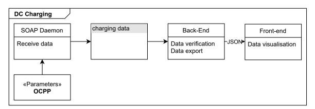
Fig. 9.3 Simplified class diagram of REView's DC station management.
