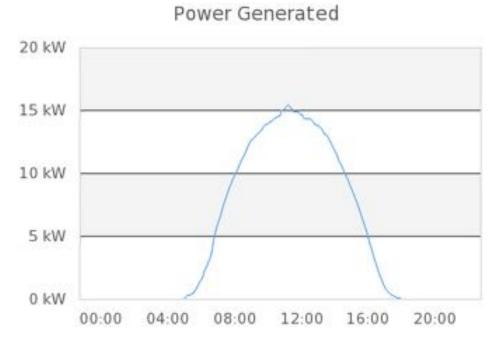
Fig. 9.29 Average power output for 20 kW of UWA's solar PV system on a given day in February.
