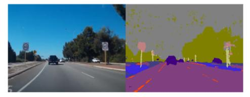
Fig. 5.7 SegNet's input (left) and output (right) for a dual carriageway in the Perth metro area.
