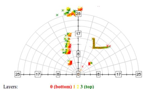
Fig. 6.3 LiDAR plot showing the detected parked vehicles at the position where Fig. 6.4 was captured. The graph axes measure distances in metres.
