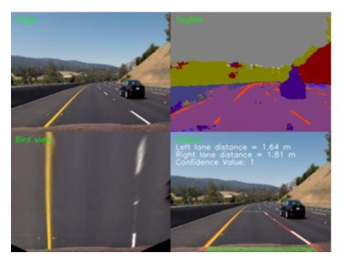
Fig. 6.7 Original and Jetson TX1 output showing segmentation, bird's eye view, vehicle distance to left and right lane marks.
