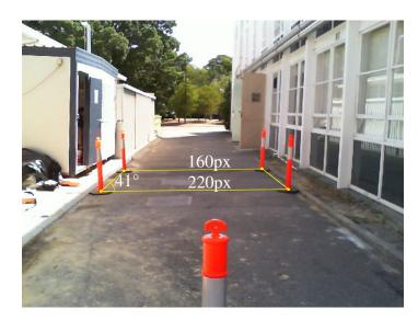
Fig. 5.5 Frame captured from the vehicle's camera for distance calibration.
