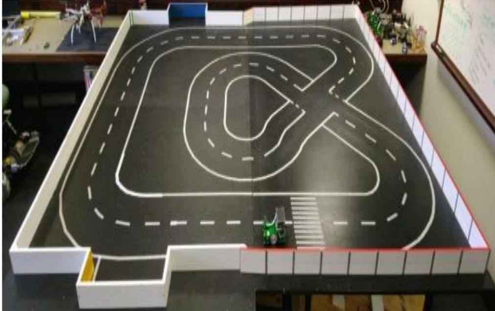
*Figure 1-4 Scaled (1:2) Carolo cup track available to train and test on in the Robotics Laboratory [12]*
