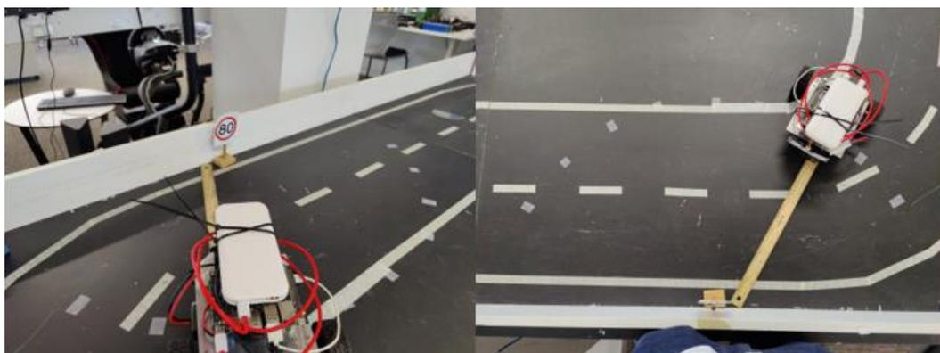
*Figure 3-18 Speed Limit Recognition test method*
