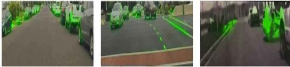
*Figure 2-3 PilotNet saliency example [27]*
