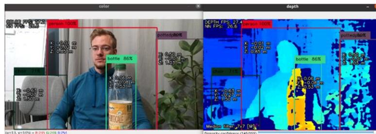
*Figure 5-1 Luxonis object detection example integrated with stereo camera to allow for detections to have their position relative to the camera estimated [66]*
