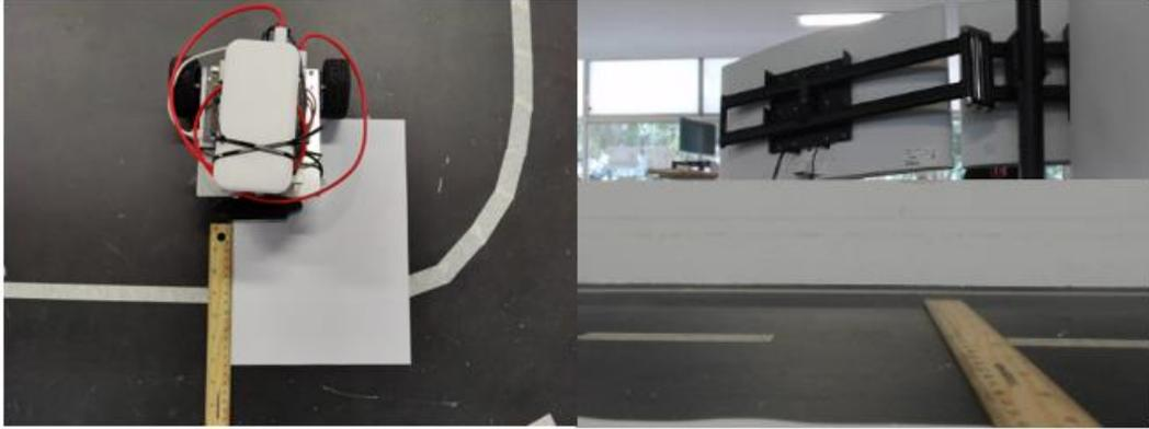
*Figure 3-3 16 cm camera dead zone based on white paper test*
