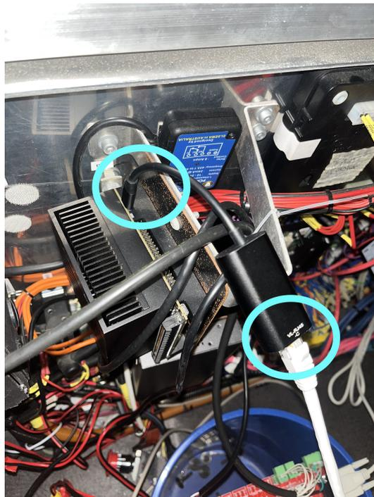
Figure 4.3: USB-C Ethernet converter utilised as a second network connection for the Jetson Xavier direct to Pointgrey camera
