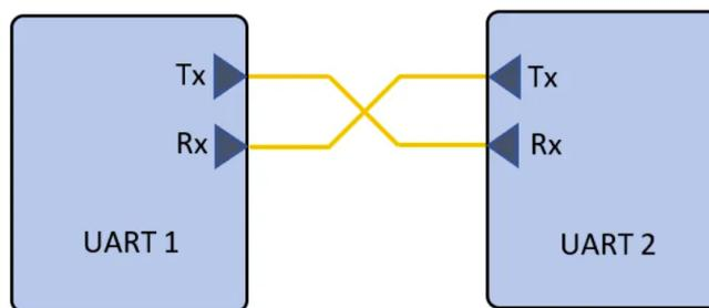
Figure 4.12: UART protocol wiring diagram. [29].
