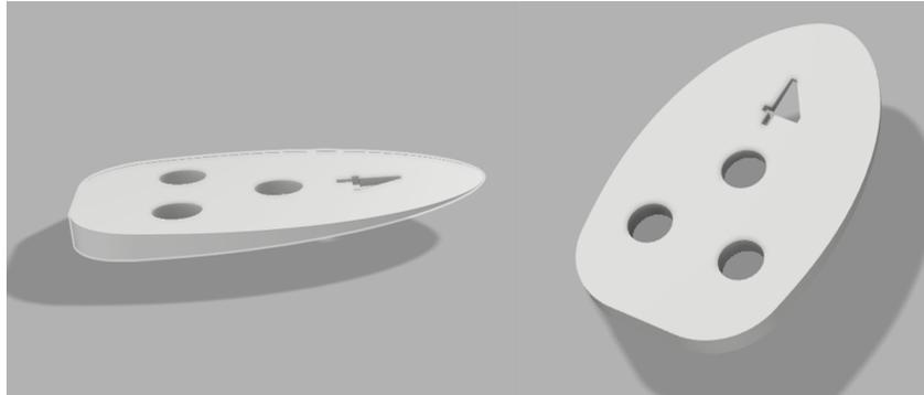
Figure 5.18: Design of offsets to adjust the angle of attack (4 degree offset).
