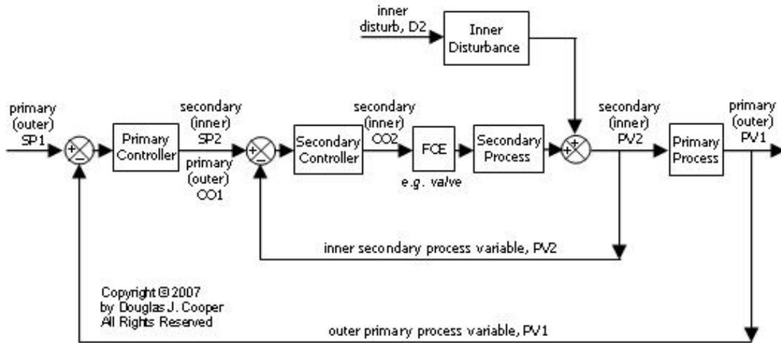
Figure 4.7: Representation of a general Cascade Controller. [24].
