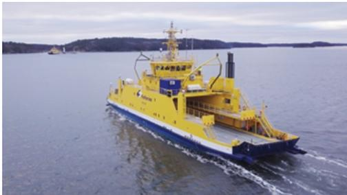
Figure 3.8: Autonomous ferry "Utrecht" Developed by Rolls Royce [14].
