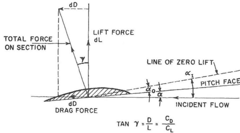
Figure 4.5: Diagram of Angle of Attack ( $\alpha$ ). [22].
