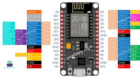
Figure 4.13: ESP8266 Module Pin-out[30].
