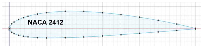
Figure 5.2: NACA 2412 Airfoil Profile
