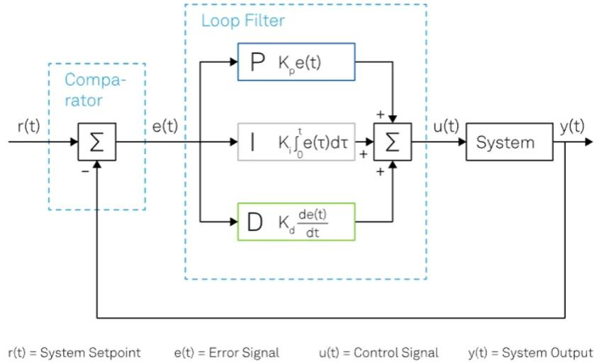
Figure 4.6: Representation of a general PID control loop in general form. [23].
