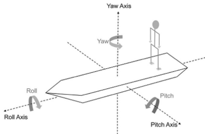
Figure 4.8: Roll, Pitch and Yaw axis of a boat. [25].
