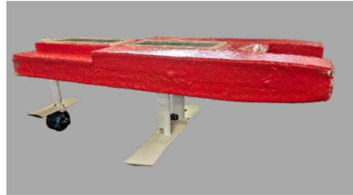
Figure 5.25: Final build of the hydrofoil (side view).
