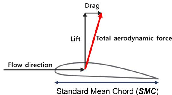
Figure 4.1: Forces Diagram of a Wing.
