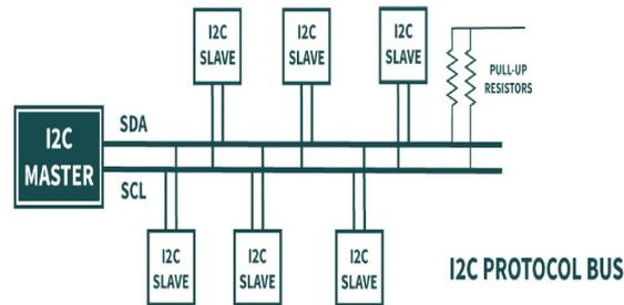
Figure 4.10: I2C protocol wiring diagram. [27].
