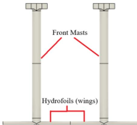
Figure 5.6: Front Mast Assembly.
