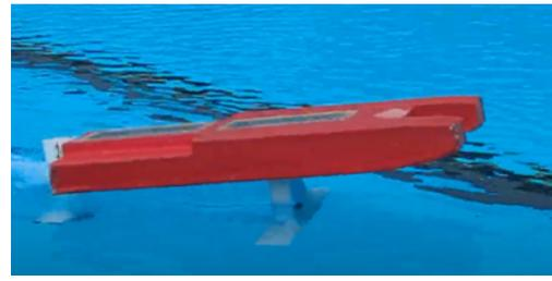
Figure 5.31: Final hydrofoil design foiling
