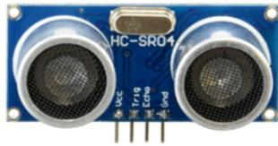
Figure 5.27: Ultrasonic sensor for distance measurement.
