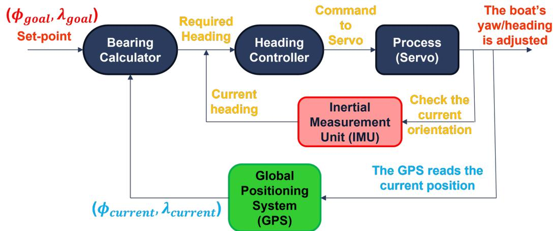
Figure 5.34: Cascade control loop for waypoint navigation
