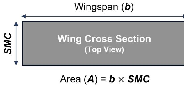
Figure 4.2: Cross-section area of a wing.
