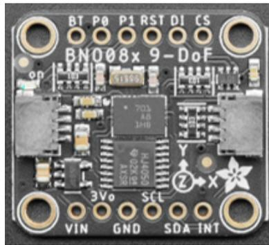
Figure 5.26: BNO085 IMU for Hydrofoil System
