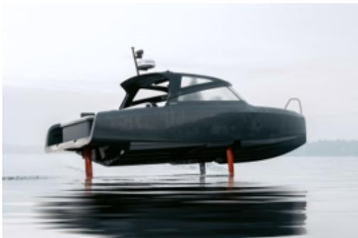
Figure 3.3: Candela C8 with hydrofoil wings[6].
