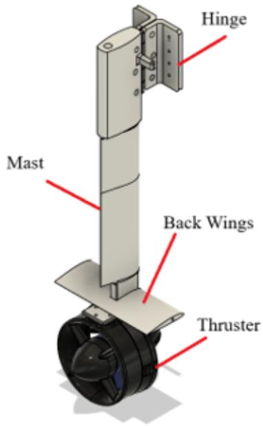
Figure 5.4: Back Mast Assembly.
