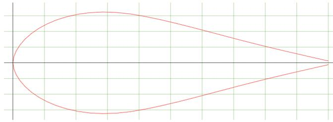
Figure 5.3: Eppler 862 Strut Wing Profile
