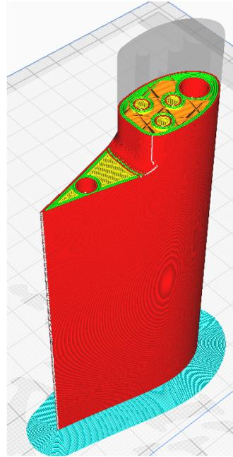
Figure 5.13: Cura Slicer - layer abstraction of model.
