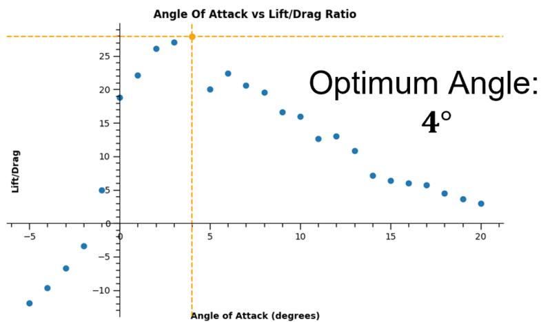
Figure 5.20: Plot to find the optimum lift/drag ratio for a given AoA.
