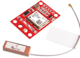
Figure 5.28: GPS module for real-time position tracking [32].
