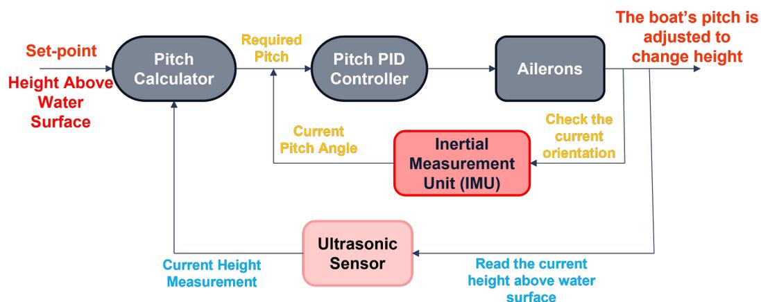
Figure 5.32: Control Feedback Loop Diagram
