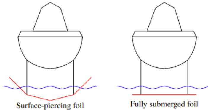
Figure 3.5: Different types of hydrofoils. Submerged (right) and Surface piercing (left).[10].
