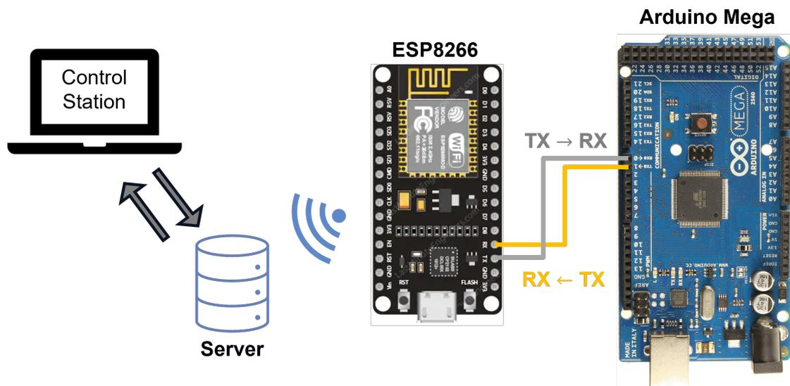
Figure 5.29: Usage of ESP8266 for Wi-Fi connectivity and web server hosting.
