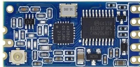
Figure 4.14: HC-12 Radio Module [31].
