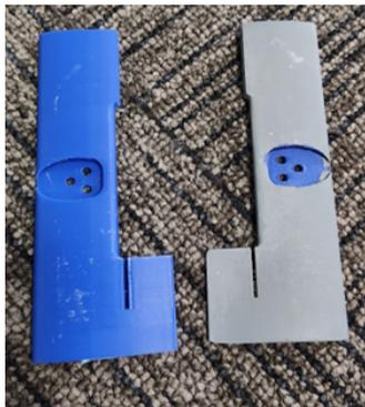
Figure 5.10: Before and After primer coating.
