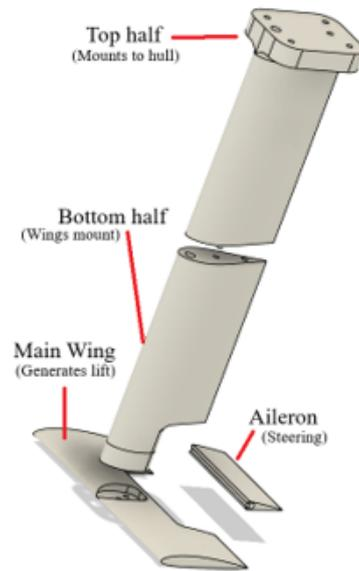
Figure 5.7: Explosion Diagram of Front Mast Assembly.
