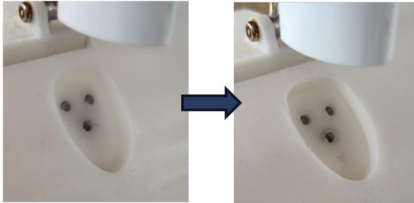
Figure 5.19: AoA offsets in place, between the mast and wing interface.
