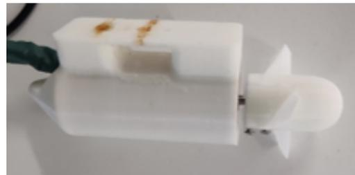
Figure 5.17: Brushless motor used as a replacement with custom propeller.
