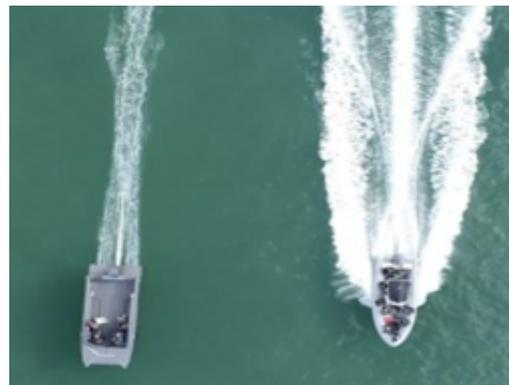
Figure 3.4: Comparison of wave trail between hydrofoil boat (left) and traditional boat (right) [7].
