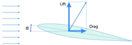
Figure 3.1: Wing Force Diagram[2].
