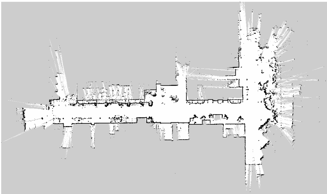
Figure 10 Map created using SLAM-Toolbox for driving tests
