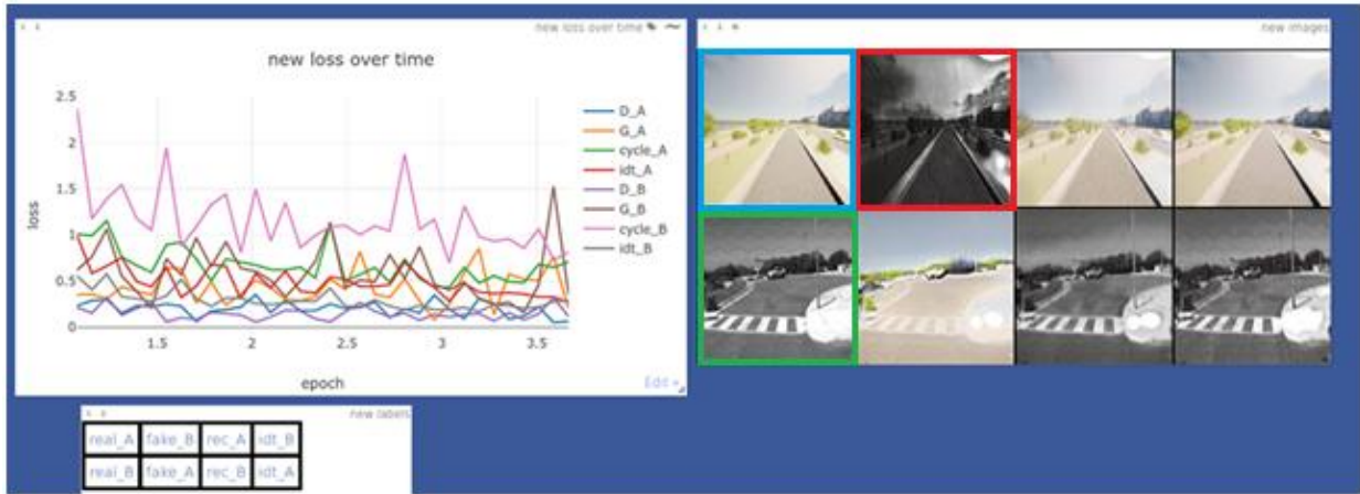
Figure 2.6: Example of early epoch Visdom monitoring during CycleGAN training. Raw CARLA (blue-box), adapted CARLA (red-box) and real image (green-box)
