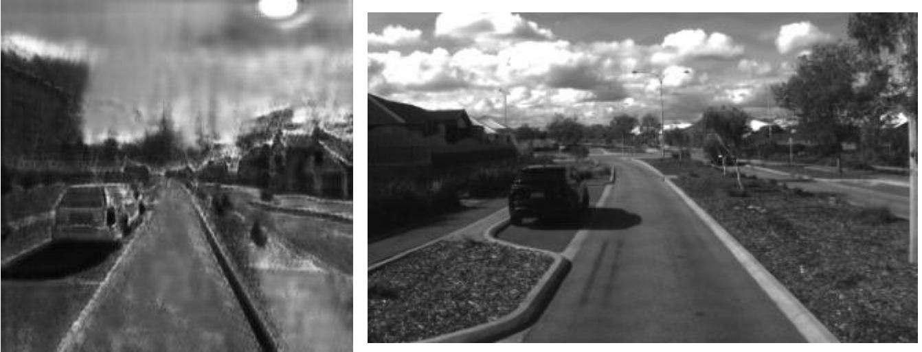
Figure 3.3: Comparison between a CycleGAN-stylized CARLA frame (left) and a real Eglinton image (right). However, infrequent textures like the mulch on the right are not in CARLA.
