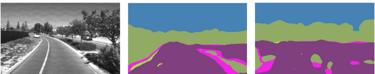
Figure 3.9: Improved model prediction comparison of GAN-adapted model (middle) with baseline model (right), showing stronger detection of road lines, curbs, land strips and adjacent roads.
