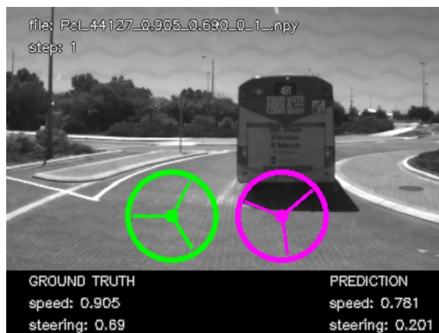
Figure 3.7: Understeering Comparing to the Ground Truth
