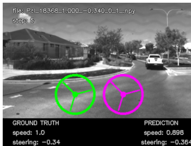
Figure 3.5: Good Alignment of Prediction with the Ground Truth
