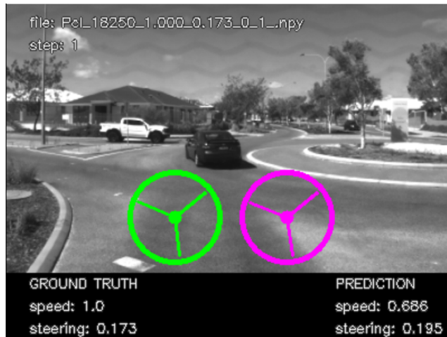
(a) Camera View. A comparison of the model’s predicted driving command (pink wheel, bottom right) against the recorded dataset’s ground truth driving command (green wheel, bottom left).
