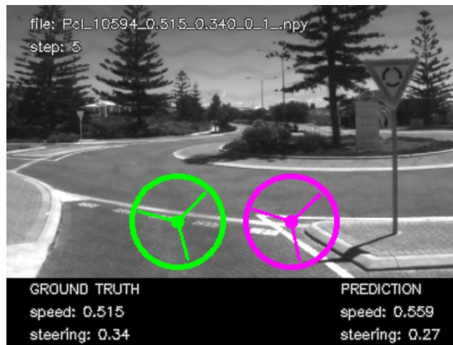
(a) Camera View. A comparison of the model’s predicted driving command (pink wheel, bottom right) against the recorded dataset’s ground truth driving command (green wheel, bottom left).
