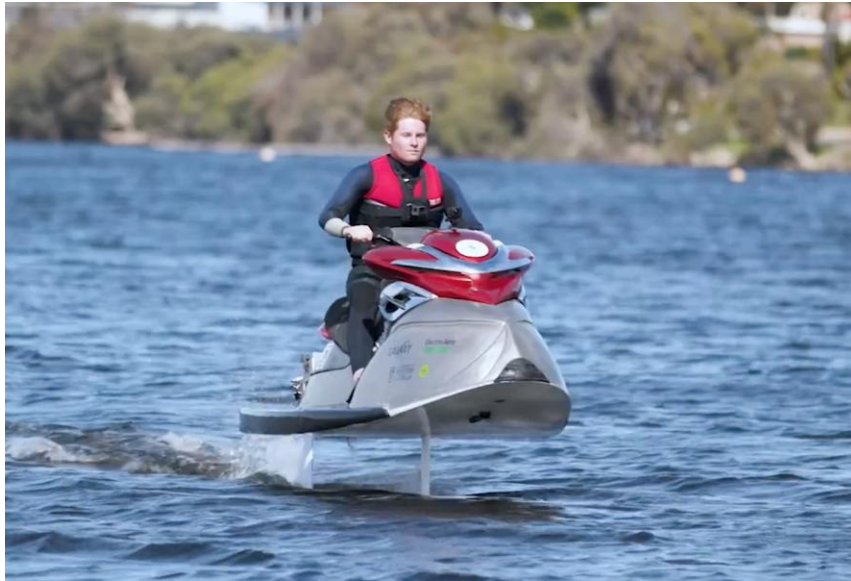
Figure 2: Electric Hydrofoil Jet-Ski Developed by the REV Project [8]
