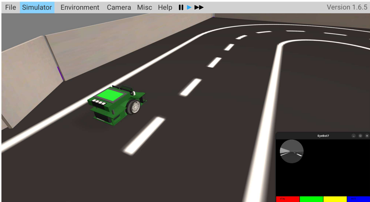
Figure 2.4: Image of an EyeBot in simulation on the Carolo Cup course, the image visible to the EyeBot is displayed on the LCD.
