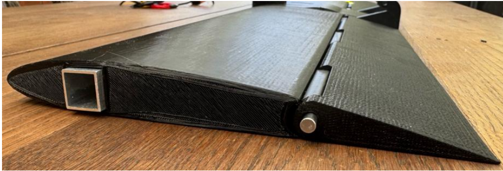
Figure 65: NACA 2412 profile with hinged aileron [16]
