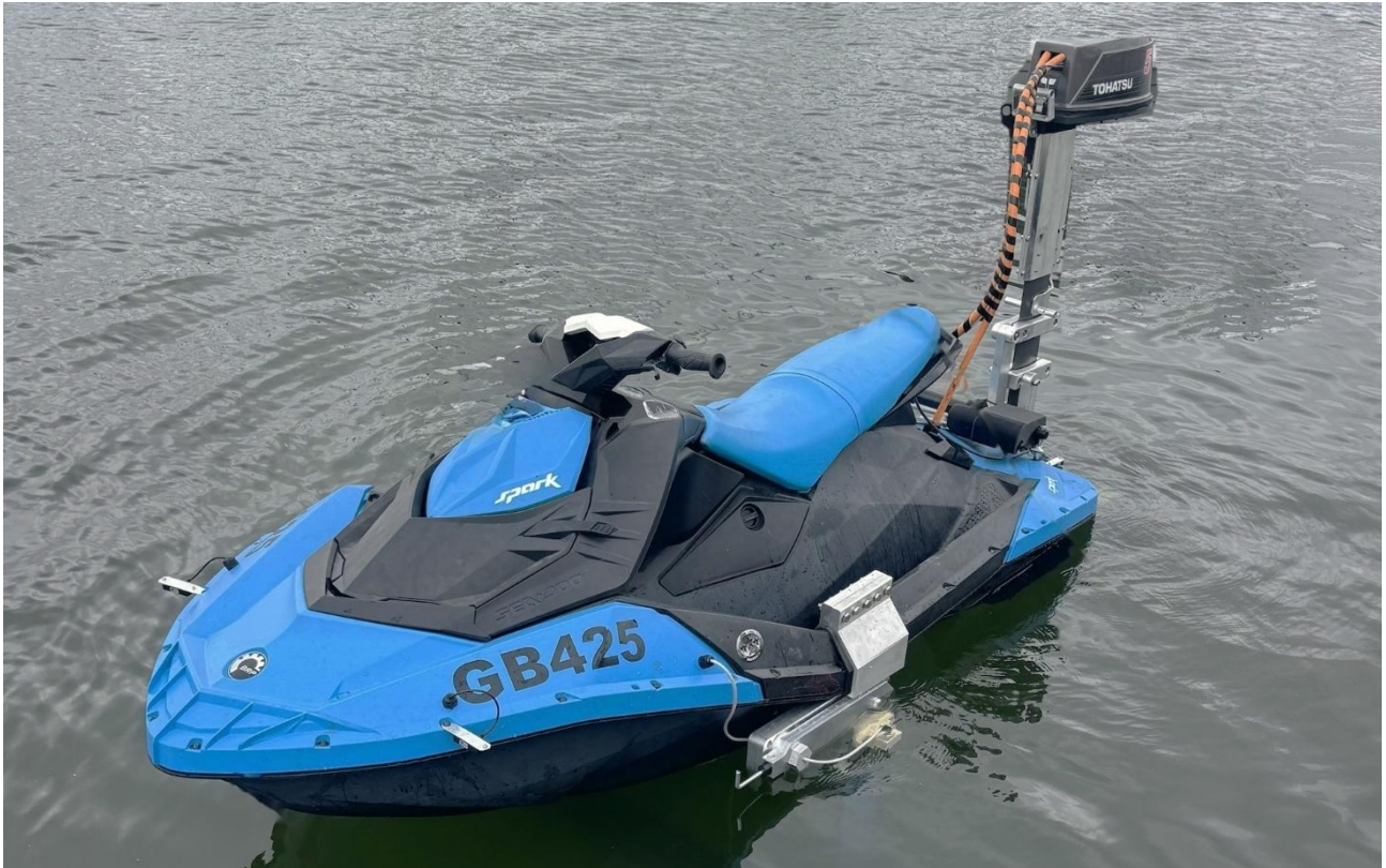
Figure 62: Initial water testing - Hydroski in deployed position
