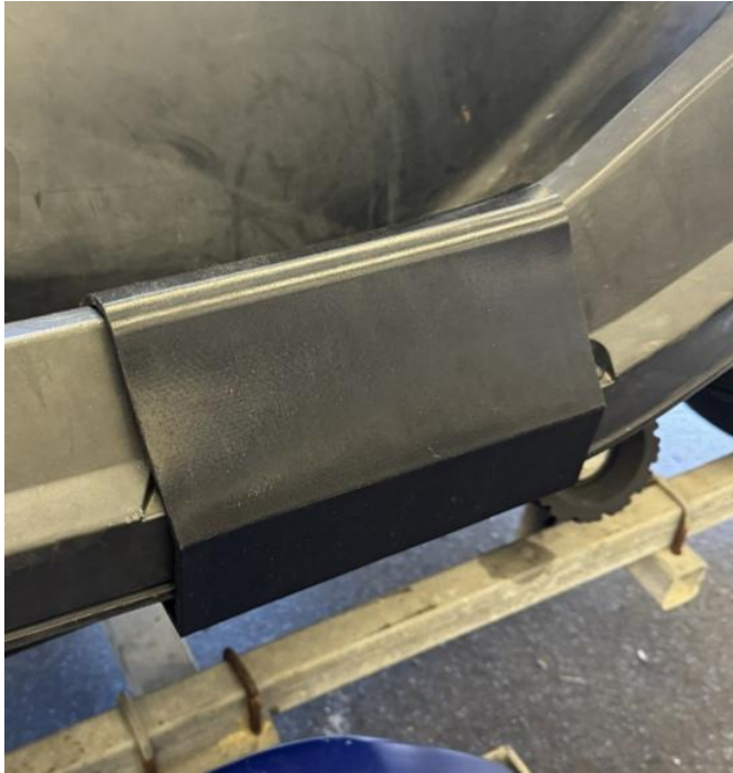
Figure 26: TPU pad over hull lip and hull clamp over pad
