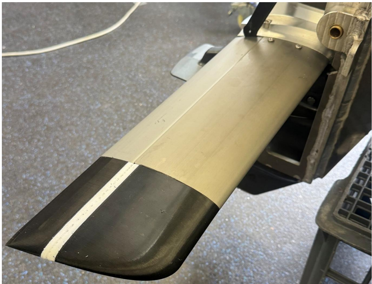
Figure 51: TPU wing prototype 2 assembled with rear foil
