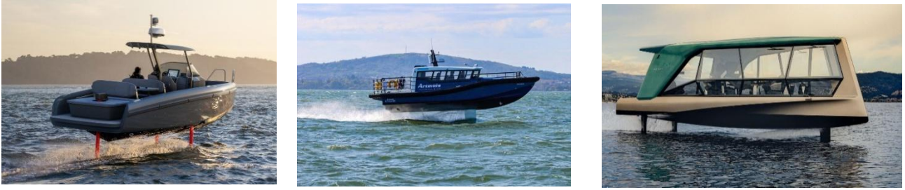
Figure 4: Fully Submerged Foils; Candela C-8, BMW Icon, Artemis e-Foiler [2] [17] [19]
