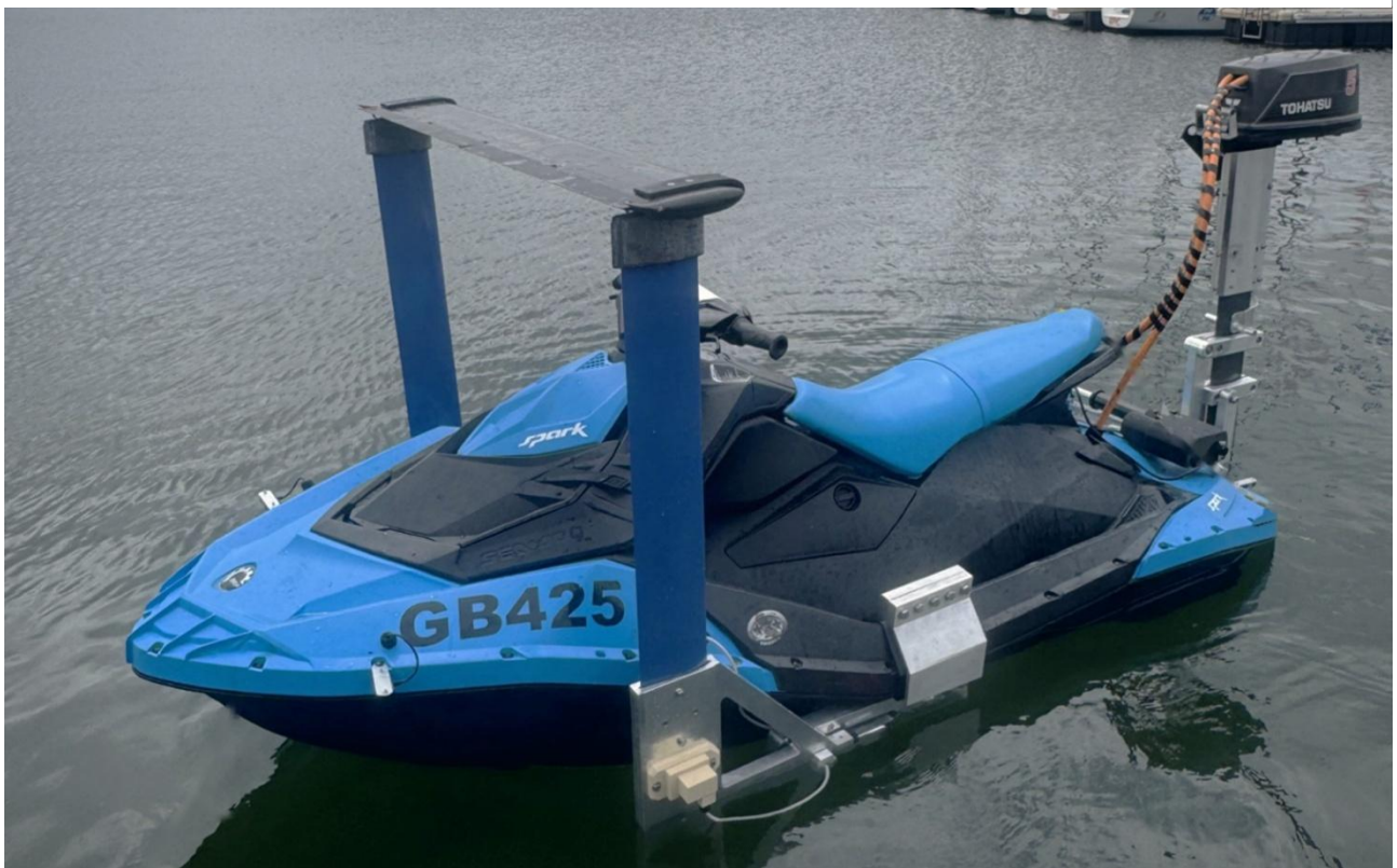
Figure 61: Initial water testing – Hydroski in retracted position
