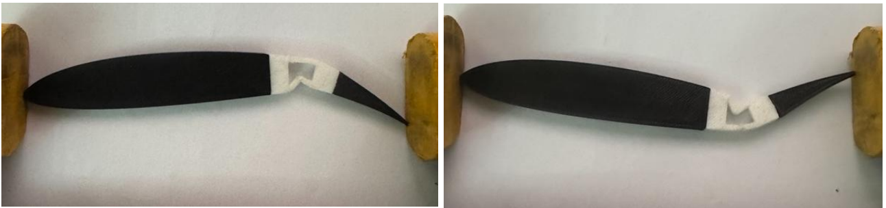
Figure 45: Test print 2 flexure test
