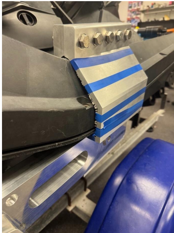
Figure 24: Hull clamp mounted with temporary rubber pad
