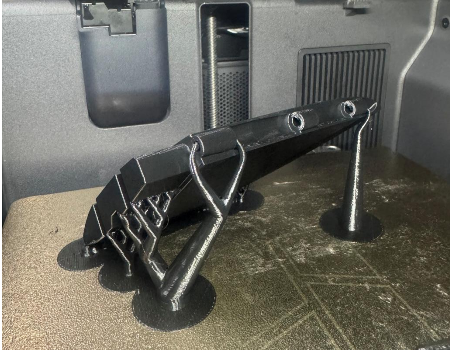
Figure 55: Recommended print orientation for wingtip
