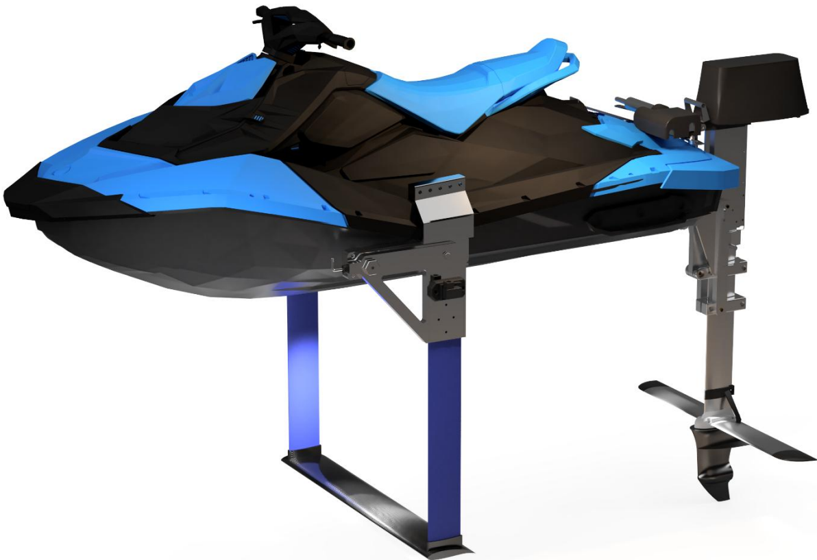
Figure 10: CAD render - Hydroski in deployed position
