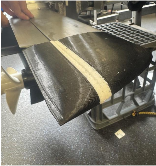
Figure 52: TPU wing prototype 2 aileron movement
