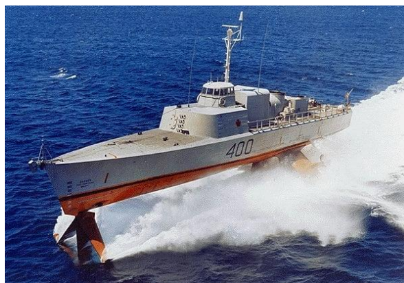
Figure 3: Surface Piercing Foil HMCS Bras d' Or [18]
